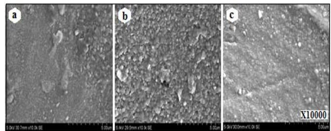
Fig. 6 SEM structure at 200mm/min (a) HAZ-Ti side (b) FZ (c) HAZ-Al side
