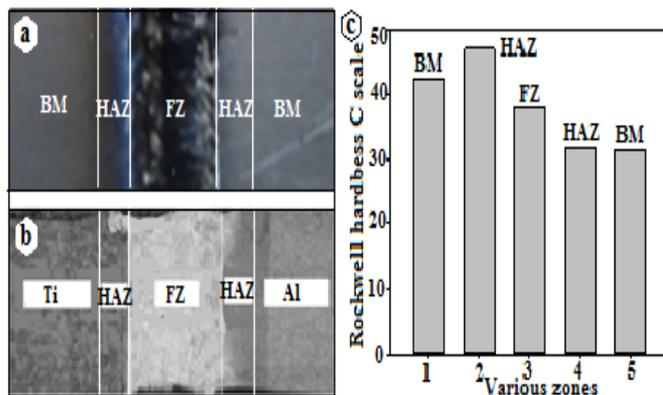
Fig. 9 (a) Various zone at weldment (b) Cross section zones (c) Hardness distributions
