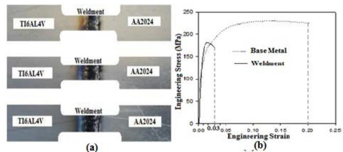
Fig. 10 (a) Test specimens (b) Stress-Strain diagram
