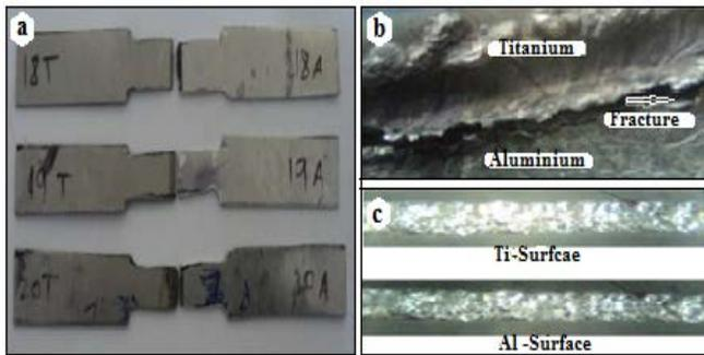
Fig. 11 (a) Fractured specimen (b) Fracture interface position (c) Fracture surface
