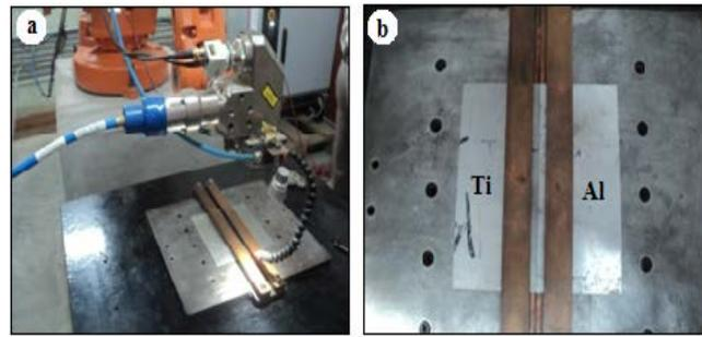
Fig.2 (a) Laser unit (b) Clamping device
