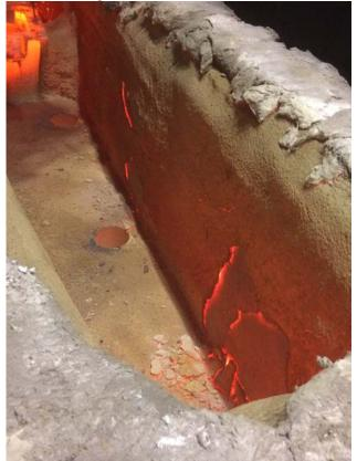
Fig. 8. Gunning mass chipping, while preheating process.
