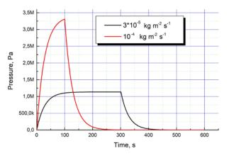
Fig. 7. Water vapor, formed of  $Mg(OH)_2$  decomposition, pressure, depending on decomposition rate.
