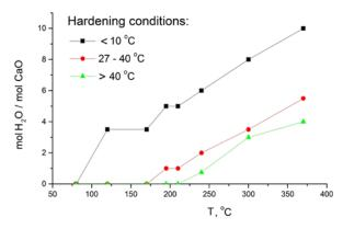
Fig. 1. Free humid formation while thermal dissociation of calcium hydro aluminates, depending on concrete hardening temperature.
