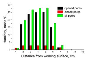
Fig. 6. Calculated humidity of lining working layer after 5 hours exposition (gunning mass was applied to the wall with surface temperature 200  $^{\circ}$ C).
