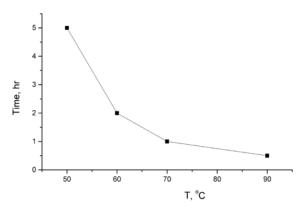
Fig. 2. "Temperature - time" map of magnesium hydroxide synthesis.
