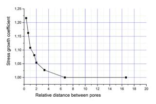
Fig. 10. Coefficient of stress growth dependence on relative distance between pores.
