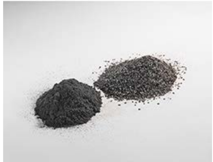
Fig. 5. SIGRATHERM GFG expanded graphite powder for enhancing thermal conductivity [26]
