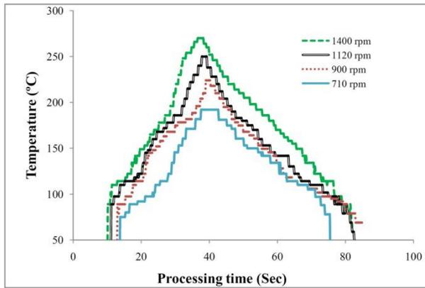
Fig. 6. Effect of the rotational speed on the temperature history experienced by material
