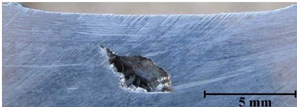
Fig. 7. Cross section of the FSPed specimen with the second tool at the rotational and traverse speeds of 710 rpm and 40 mm/min, respectively
