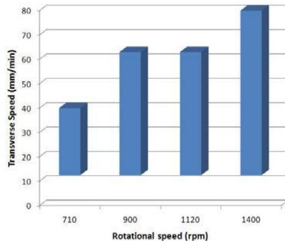
Fig 5- Acceptable traverse speed range versus the rotational speeds in the FSP by the first tool
