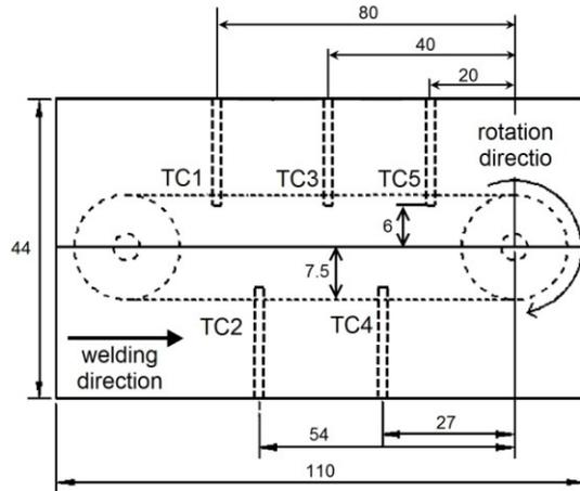
Fig. 1. Layout of the thermocouples inside the work piece.
