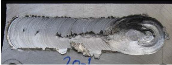
Fig. 3. Surface of the specimen FSPed by the first tool at the rotational and traverse speeds of 710 rpm and 63 mm/min, respectively
