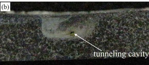
Fig. 4. (a) Surface of the FSPed specimen by the first tool at the rotational and traverse speeds of 1400 rpm and 100 mm/min, respectively and (b) etched cross section of the specimen of Fig. 4a.
