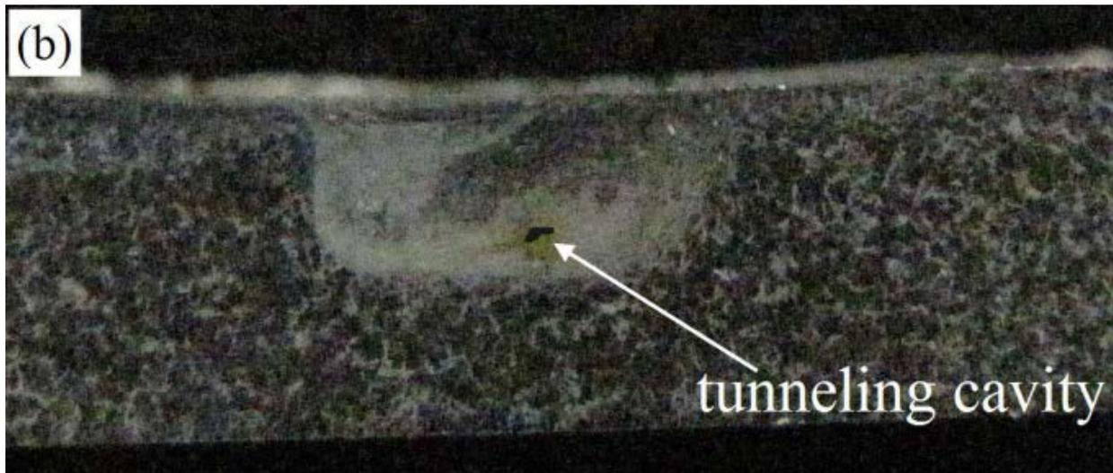
Fig. 4. (a) Surface of the FSPed specimen by the first tool at the rotational and traverse speeds of 1400 rpm and 100 mm/min, respectively and (b) etched cross section of the specimen of Fig. 4a.
