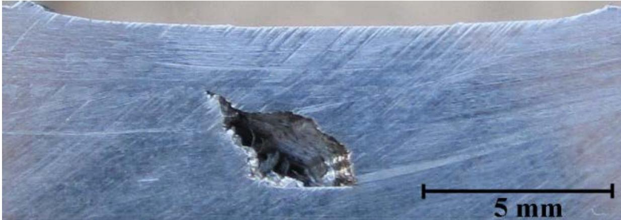
Fig. 7. Cross section of the FSPed specimen with the second tool at the rotational and traverse speeds of 710 rpm and 40 mm/min, respectively
