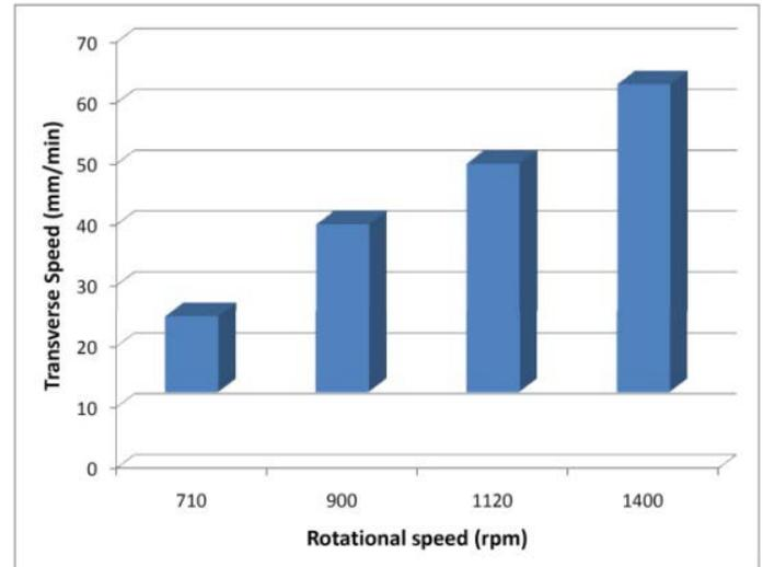
Fig. 8. Acceptable traverse speed range versus the rotational speeds in the FSP by the second tool
