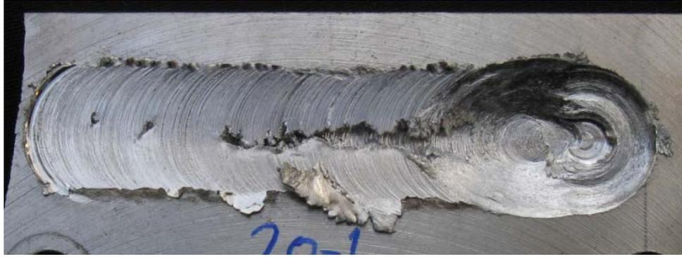
Fig. 3. Surface of the specimen FSPed by the first tool at the rotational and traverse speeds of 710 rpm and 63 mm/min, respectively
