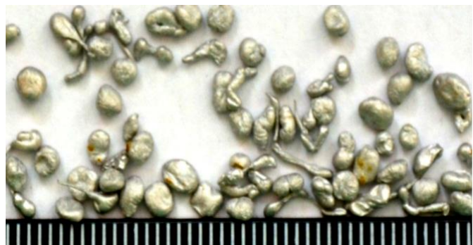
Fig. 13 particles of aluminum produced on centrifugal granulator
