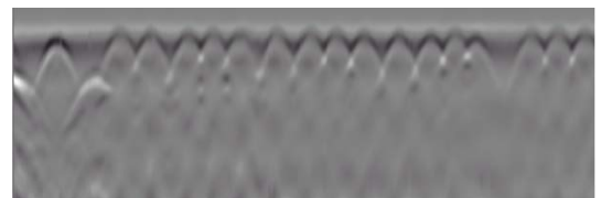
Fig.16-a The relatively sound concrete area with its radar profile
