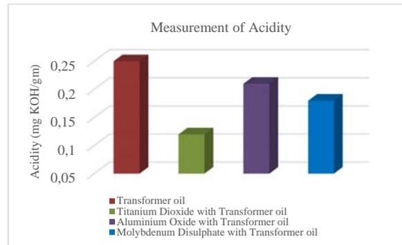
Figure 5. Graphical comparison of acidity between the transformer oil and nanofluids based transformer oil (in mgKOH/gm).
