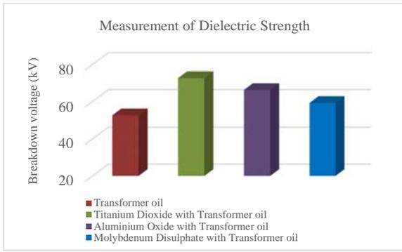
Figure 4. Graphical comparison of dielectric strength between the transformer oil and nanofluids based transformer oil (in kV).
