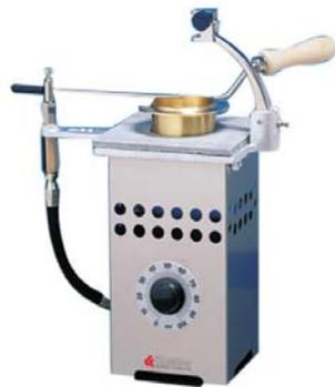
**Figure 7.** Schematic diagram of cleaveland open cup flash point tester.
