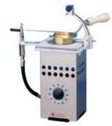
Figure 7. Schematic diagram of cleaveland open cup flash point tester.
