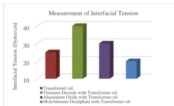
Figure 6. Graphical comparison of interfacial tension between the transformer oil and nanofluids based transformer oil (in Dynes/cm).
