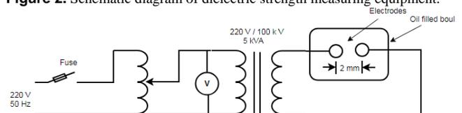
Figure 3. Circuit diagram of dielectric strength test
