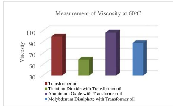
Figure 13. Graphical comparison of dynamic viscosity between the transformer oil and nanofluids based transformer oil at 60°C.
