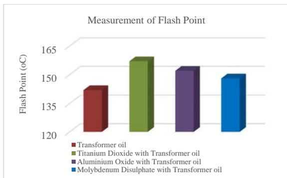
**Figure 8.** Graphical comparison of flash point between the transformer oil and nanofluids based transformer oil (in °C).
