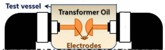
Figure 1. Schematic diagram of front view of dielectric strength measuring equipment.
