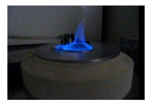
Figure 9. Blue flame produced in transformer oil.
