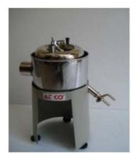
Figure 11. Schematic diagram of red wood viscometer.
