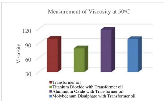
Figure 12. Graphical comparison of dynamic viscosity between the transformer oil and nanofluids based transformer oil at 50°C.
