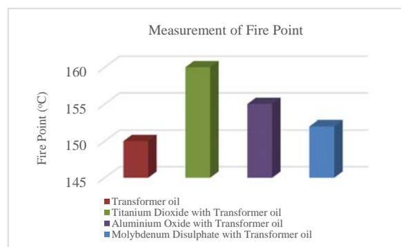
**Figure 10.** Graphical comparison of fire point between the transformer oil and nanofluids based transformer oil (in °C).
