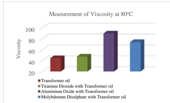
Figure 15. Graphical comparison of dynamic viscosity between the transformer oil and nanofluids based transformer oil at 80°C.
