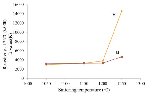
Fig.7. The resistivity and B value of sintered sample vs. the sintering temperature.
