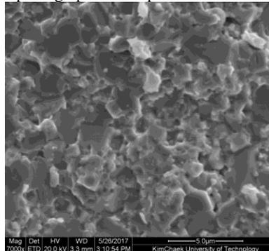
Fig.6. SEM photograph of the specimen sintered at 1250°C
