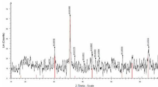
Fig.2. X-ray diffractogram of powder after firing at 800°C
