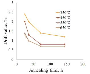
Fig.8. The drift value vs. the annealing temperature and time.
