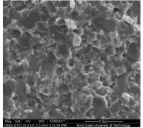
Fig.6.SEM photograph of the specimen sintered at 1 250°C
