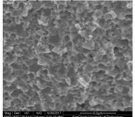
Fig.5.SEM photograph of the specimen sintered at 1 200°C
