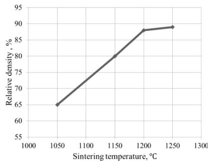
Fig. 1. The relationship between relative density and sintering temperature
