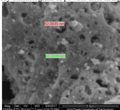
Fig.3. SEM photograph of specimen pre-sintered at 800°C
