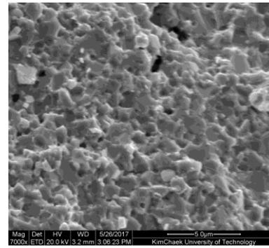
Fig.4. SEM photograph of the specimen sintered at 1050°C
