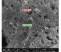
Fig.3. SEM photograph of specimen pre-sintered at 800°C
