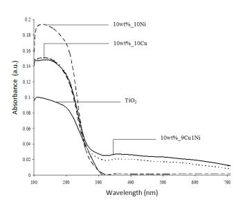
Fig. 4. DRUV-Vis spectra of the photocatalysts.
