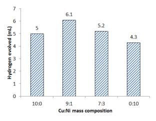
Fig. 5. The effect of Cu:Ni mass composition of photocatalyst with 10wt% total metal loading on hydrogen production.
