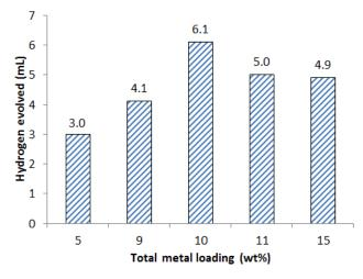
Fig. 6. The effect of total metal loading of photocatalyst (Cu:Ni mass composition 9:1) on hydrogen production.
