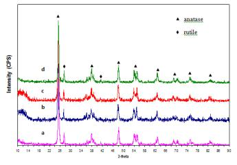
Fig. 2. XRD patterns of (a) TiO<sub>2</sub>, (b) 10wt%\_9Cu1Ni, (c) 10wt%\_10Cu and (d) 10wt%\_10Ni
