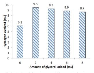
Fig. 7. The effect of glycerol amount on hydrogen production using 10wt%\_9Cu1Ni.
