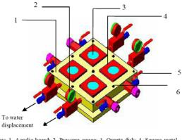
Key: 1. Acrylic board; 2. Pressure gauge; 3. Quartz disk; 4. Square metal plate; 5. One way valve; 6. Screw
