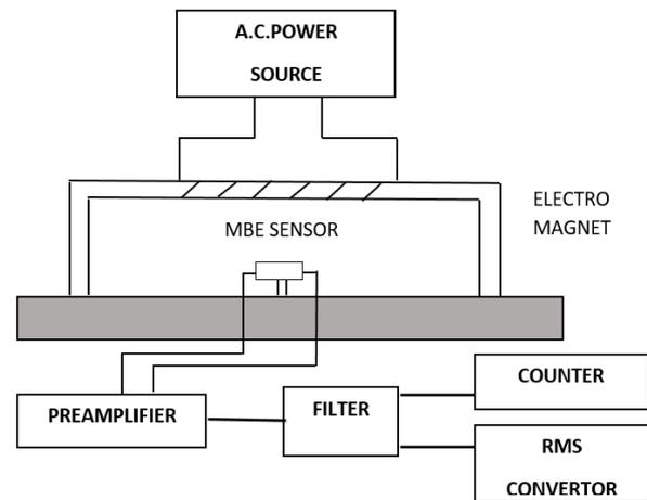
Figure 1. Block diagram of the experimental MBE – setup.
