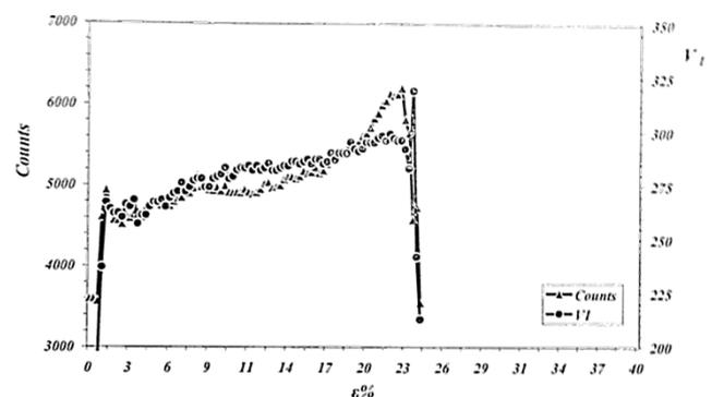
Figure 4. Plot of the Barkhausen emission signal of counts and volts respectively.
