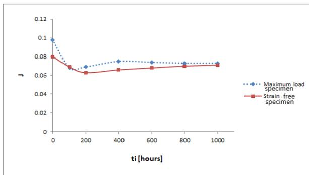
Figure 10. Magnetic  $J$ -parameter evaluation with time of corrosion.
