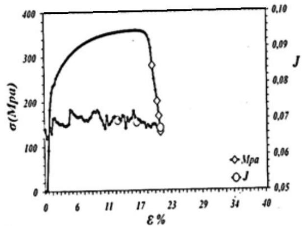
Figure 8. Mechanical stress-strain and magnetic  $J$ -response curves for 800 hours of corrosion time.
