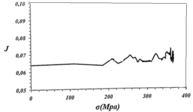
Figure 12. Stress-mode of presentation of  $J$ -parameter for 200 hours of corrosion.
