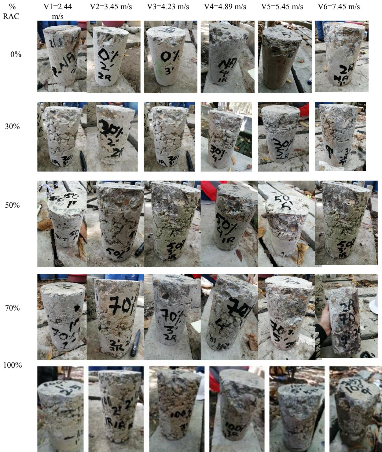
Fig. 9. Failure modes exhibited by specimens under increasing velocities
