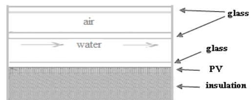
Fig. 2. Descriptive scheme for a solar photovoltaic thermal (PV/T) water collector
