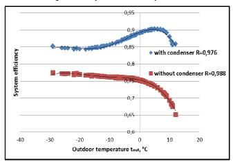
Fig. 5. Changes in heating system efficiency depending on outdoor temperature.
