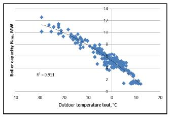
Fig. 4. Changes in boiler capacity depending on outdoor temperature.
