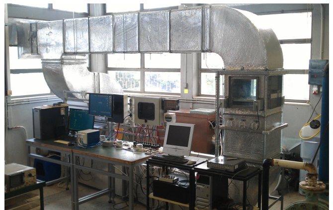
Fig. 2 Photo of the lab-scale BTA dryer, equipped with measuring instrumentation and data acquisition system
