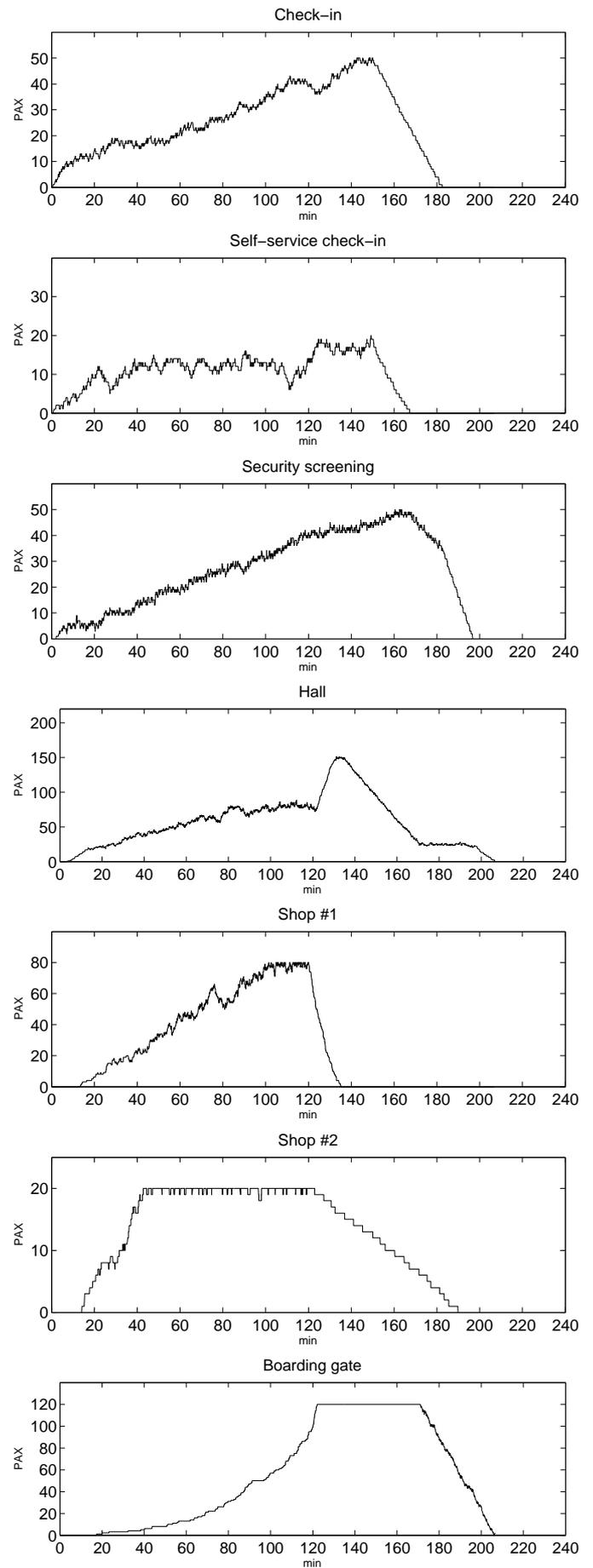
Fig. 11. Cell occupancy according to the Petri net model
