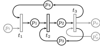
Fig. 4. Petri net model of the check-in counters
