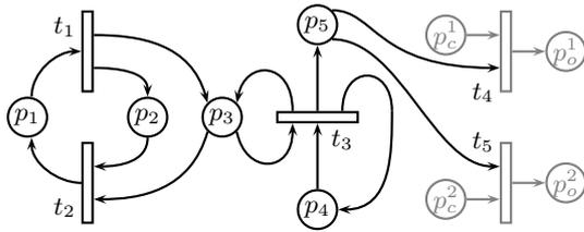
Fig. 3. Petri net model of the generator
