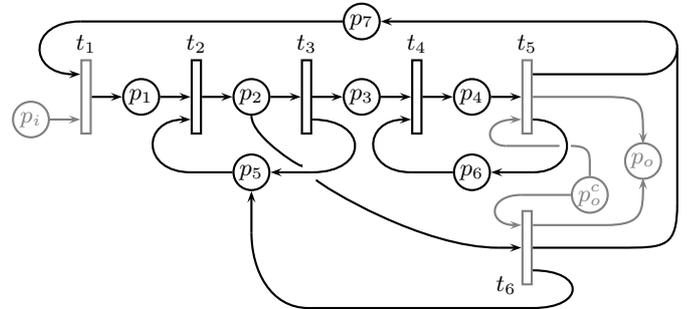
Fig. 5. Petri net model of the self-service check-in area
