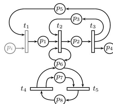
Fig. 9. Petri net model of the boarding gate
