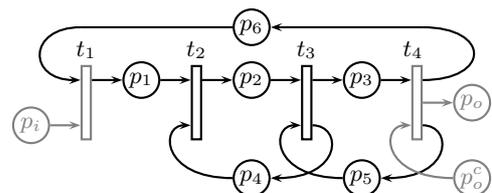
Fig. 6. Petri net model of security screening
