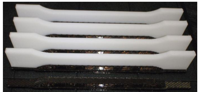
Fig. 9 Testing sample (for tensile tests) production (FDM – longitudinal position)
