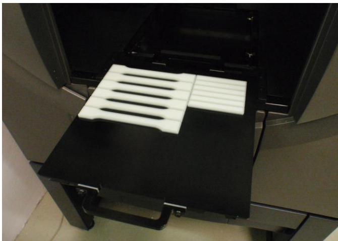
Fig. 7 Testing sample (for tensile tests) production (3D printing - PolyJet)
