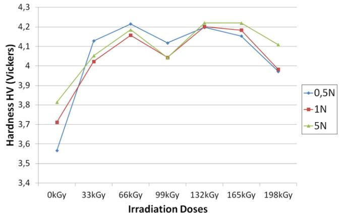
Fig. 24 Hardness Vickers of HDPE vs. irradiation doses
