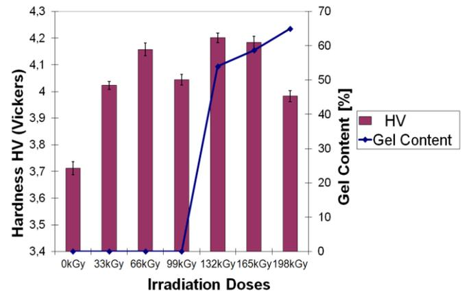
Fig. 15 Hardness Vickers of HDPE vs. irradiation doses
