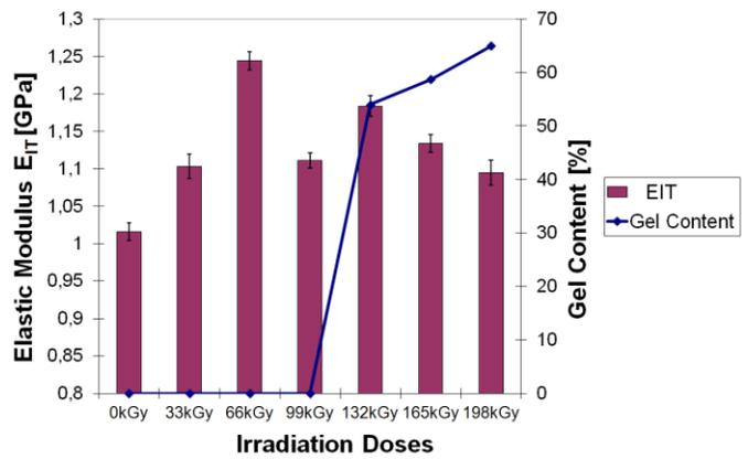
Fig. 10 Elastic modulus EIT of HDPE vs. irradiation doses
