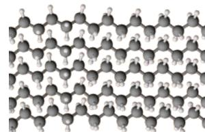
Fig. 1 Molecule structure of HDPE
