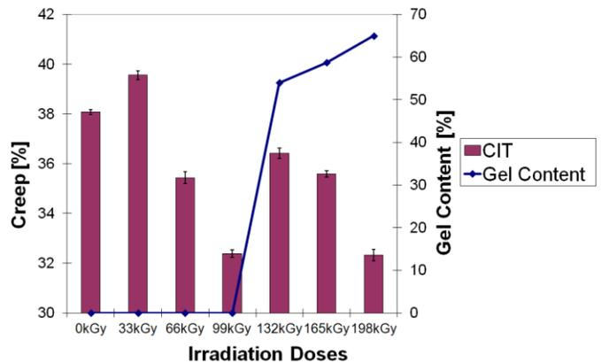
Fig. 29 Creep of HDPE vs. irradiation doses
