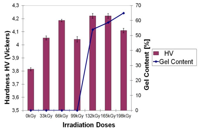
Fig. 19 Hardness Vickers of HDPE vs. irradiation doses
