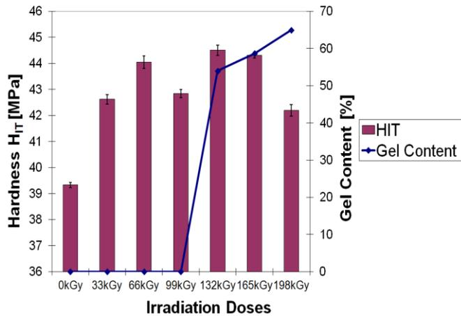
Fig. 13 Hardness HIT of HDPE vs. irradiation doses
