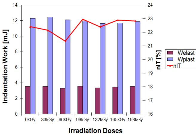
Fig. 16 Elastic and plastic deformation work of HDPE vs. irradiation dose
