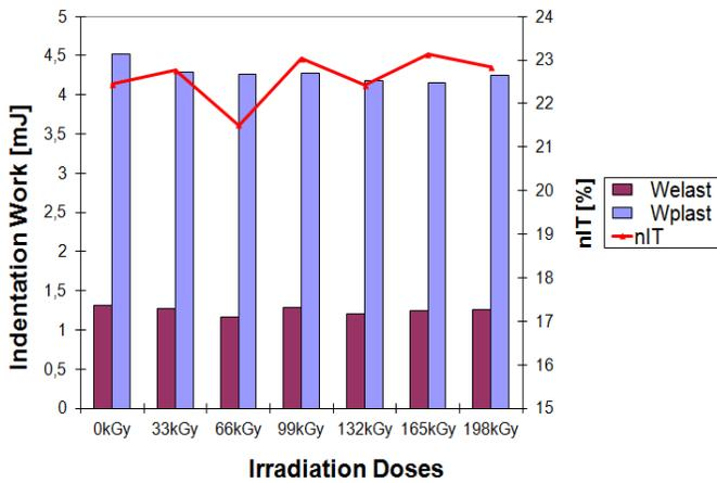
Fig. 12 Elastic and plastic deformation work of HDPE vs. irradiation dose
