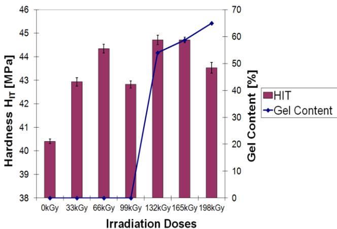
Fig. 17 Hardness HIT of HDPE vs. irradiation doses
