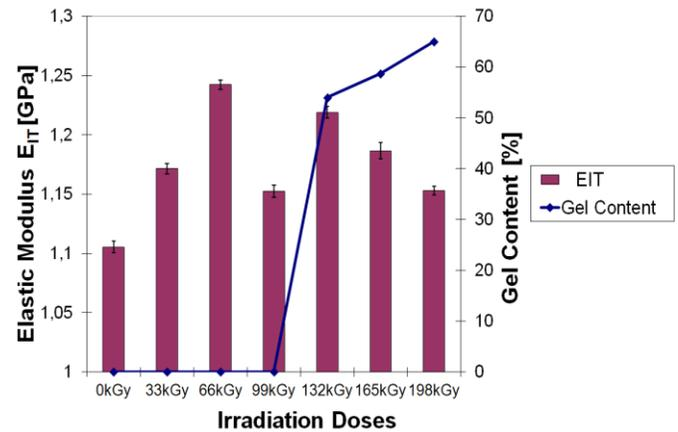
Fig. 18 Elastic modulus EIT of HDPE vs. irradiation doses
