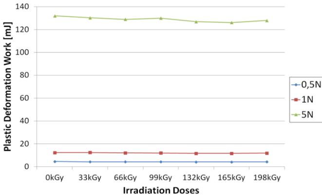
Fig. 26 Plastic deformation work of HDPE vs. irradiation dose
