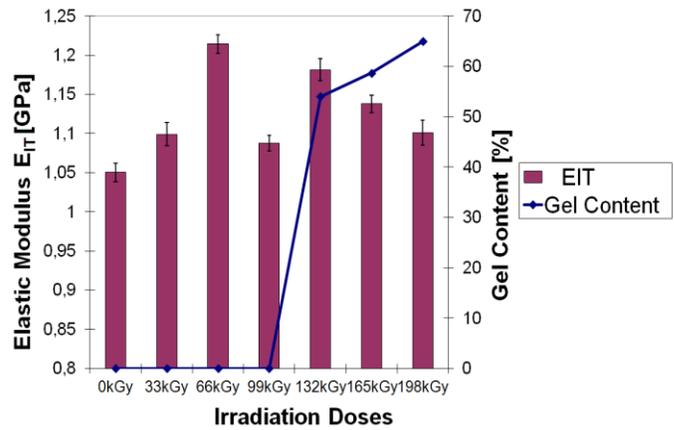
Fig. 14 Elastic modulus EIT of HDPE vs. irradiation doses
