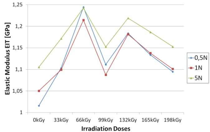
Fig. 23 Elastic modulus EIT of HDPE vs. irradiation doses
