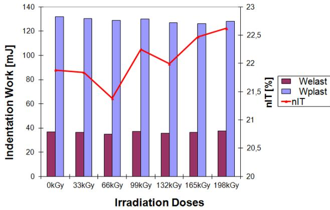
Fig. 20 Elastic and plastic deformation work of HDPE vs. irradiation dose
