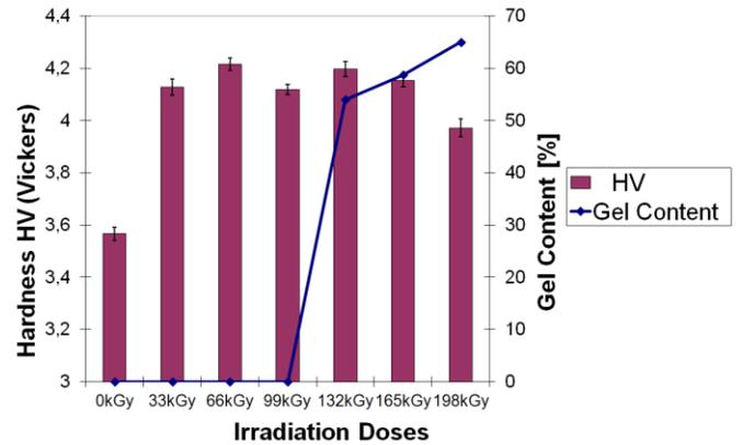
Fig. 11 Hardness Vickers of HDPE vs. irradiation doses
