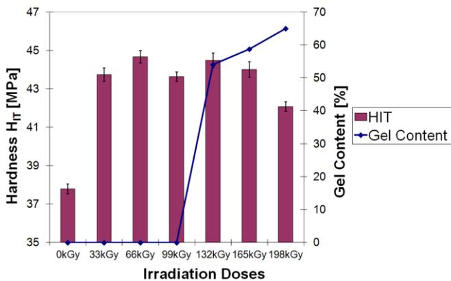
Fig. 9 Hardness HIT of HDPE vs. irradiation doses
