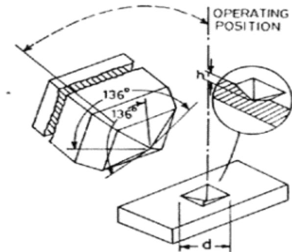
Fig. 3 The basic principle of hardness testing according to Vickers
