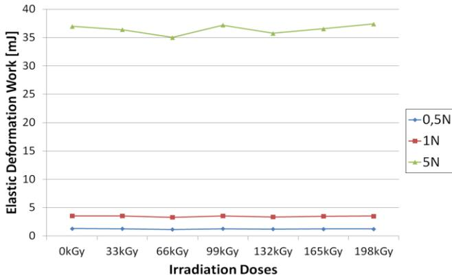
Fig. 25 Elastic deformation work of HDPE vs. irradiation dose
