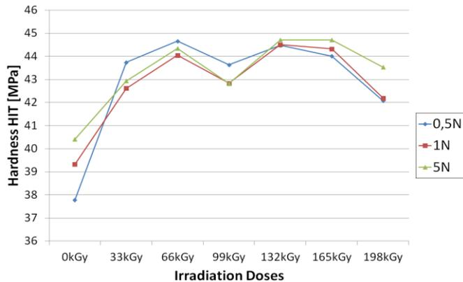
Fig. 22 Hardness HIT of HDPE vs. irradiation doses
