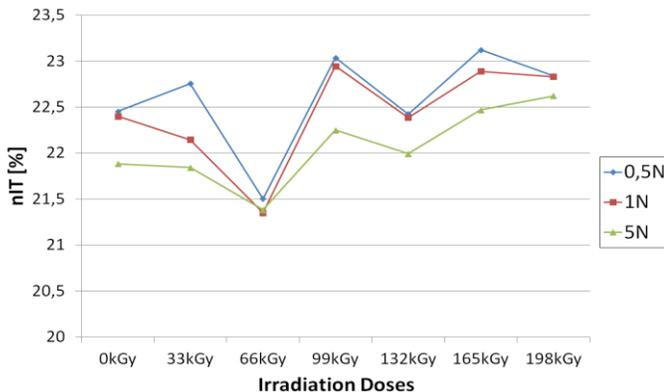
Fig. 27 Elastic part deformation work of HDPE vs. irradiation dose
