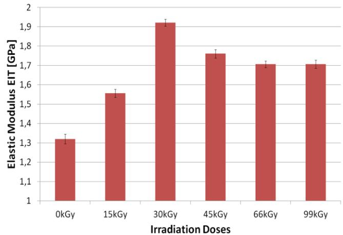
Fig. 17 Elastic modulus EIT of PA6 vs. irradiation doses
