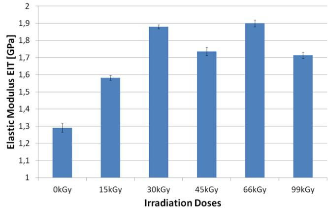
Fig. 9 Elastic modulus EIT of PA6 vs. irradiation doses
