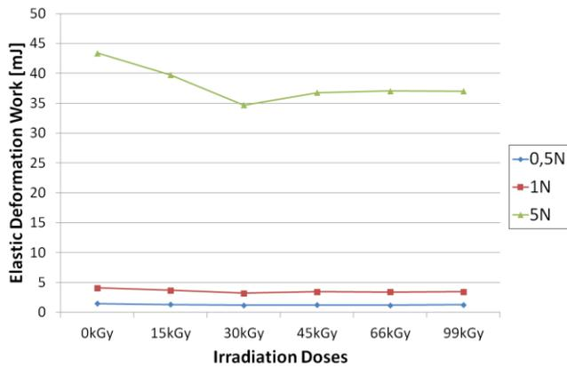
Fig. 24 Elastic deformation work of PA6 vs. irradiation dose
