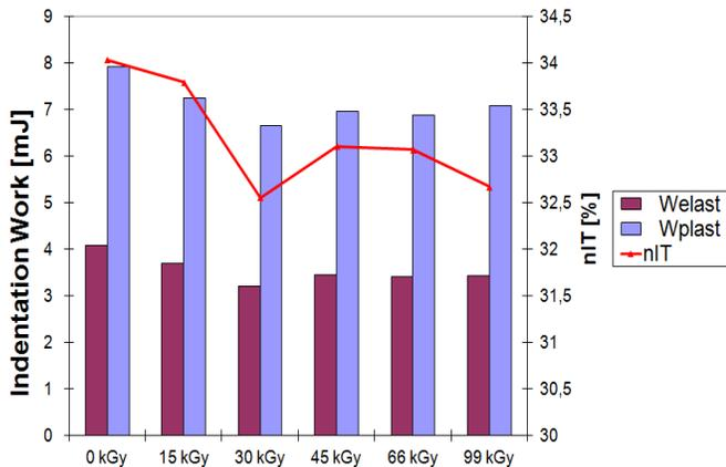
Fig. 15 Elastic and plastic deformation work of PA6 vs. irradiation dose
