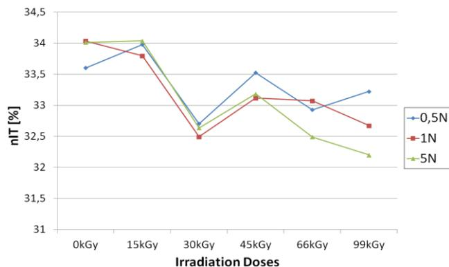
Fig. 26 Elastic part deformation work of PA6 vs. irradiation dose
