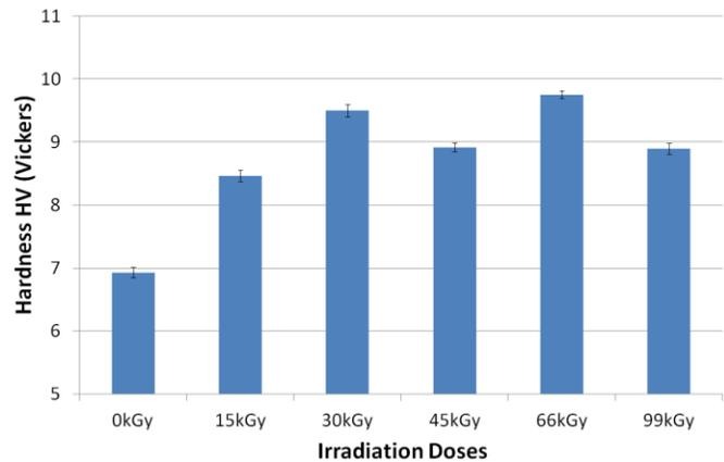
Fig. 10 Hardness Vickers of PA6 vs. irradiation doses
