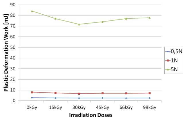
Fig. 25 Plastic deformation work of PA6 vs. irradiation dose
