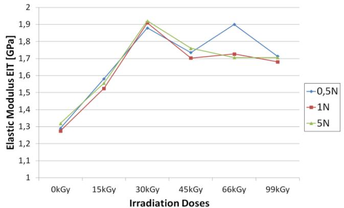
Fig. 22 Elastic modulus EIT of PA6 vs. irradiation doses
