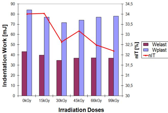
Fig. 19 Elastic and plastic deformation work of PA6 vs. irradiation dose
