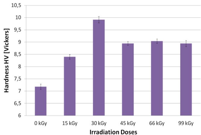
Fig. 14 Hardness Vickers of PA6 vs. irradiation doses
