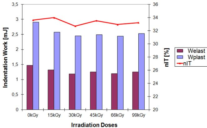
Fig. 11 Elastic and plastic deformation work of PA6 vs. irradiation dose
