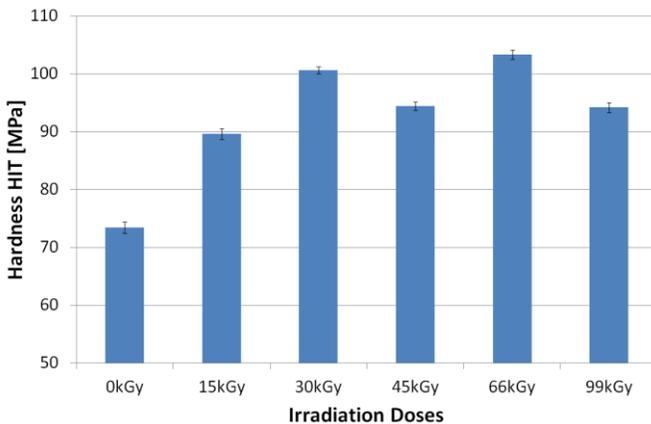
Fig. 8 Hardness HIT of PA6 vs. irradiation doses
