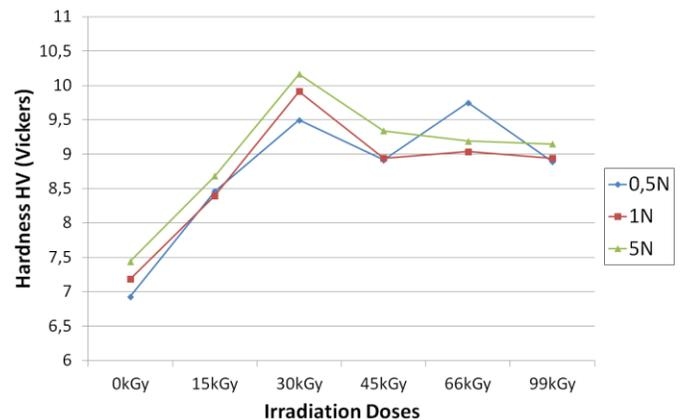
Fig. 23 Hardness Vickers of PA6 vs. irradiation doses
