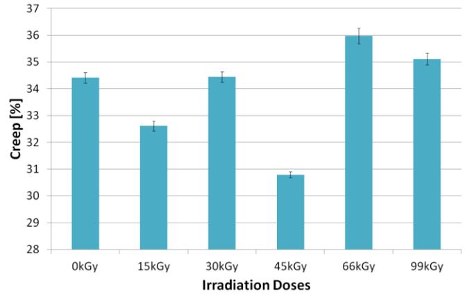
Fig. 27 Creep of PA6 vs. irradiation doses
