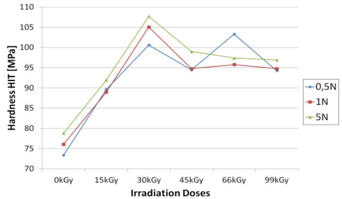
Fig. 21 Hardness HIT of PA6 vs. irradiation doses
