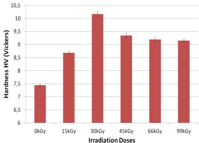
Fig. 18 Hardness Vickers of PA6 vs. irradiation doses
