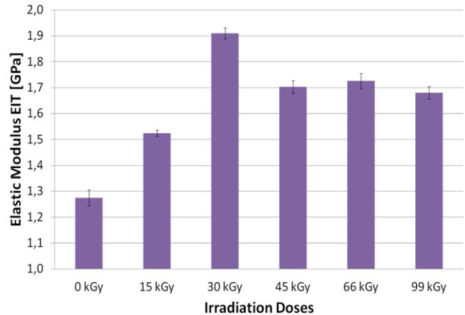
Fig. 13 Elastic modulus EIT of PA6 vs. irradiation doses
