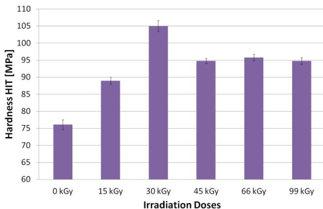
Fig. 12 Hardness HIT of PA6 vs. irradiation doses
