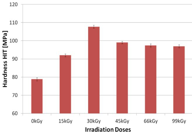
Fig. 16 Hardness HIT of PA6 vs. irradiation doses
