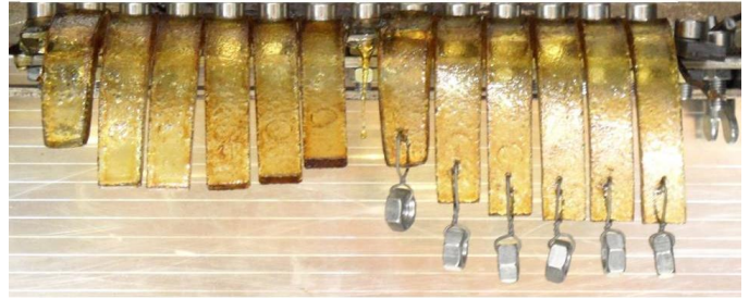
Fig. 24 LDPE specimen deformation at 220°C
