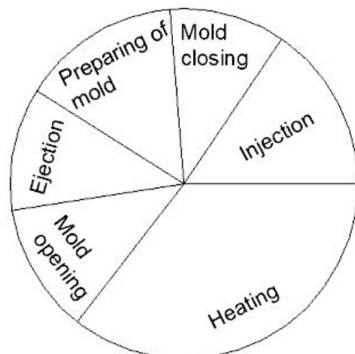
Fig. 1 Rubber injection molding cycle
