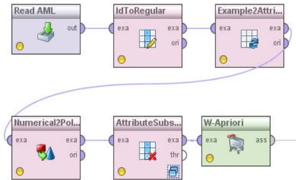
Fig. 1. Generating association rules by using the W-Apriori algorithm
