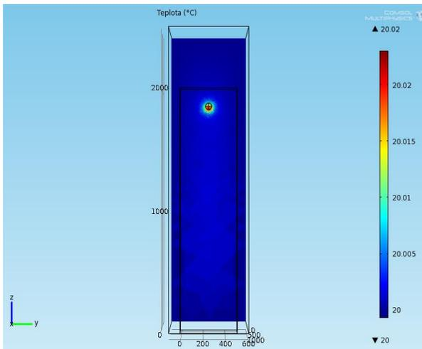
Fig. 4 The temperature distribution in the cross-sectional surface at the site of a pyroelectric element for 1 m
