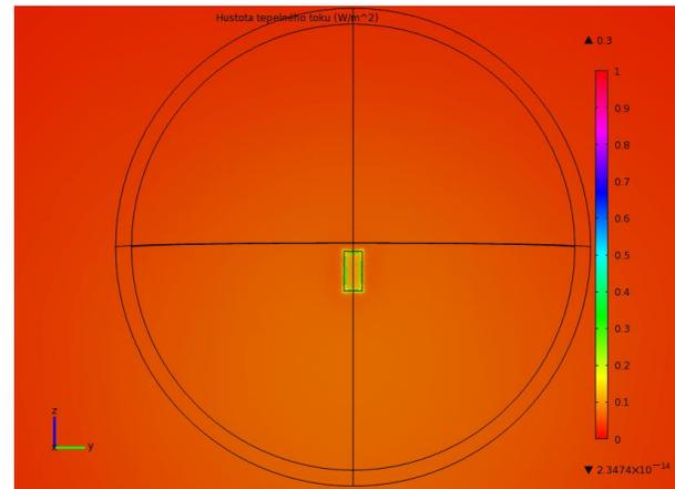
Fig. 11 The distribution density of the heat flow at the site of the cut surface of the pyroelectric element - detail in the place of the detector
