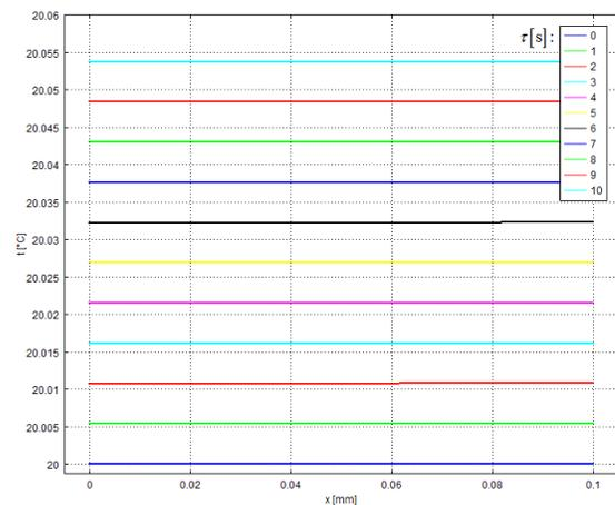
Fig. 20 Temperature field in pyroelement for the heat of the action 10 seconds calculated in COMSOL Multiphysics
