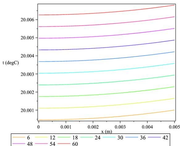
Fig. 2 2D temperature field in a heated sensor calculated in Maple
