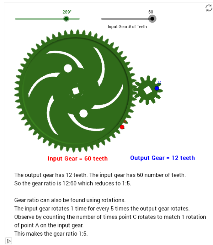
Fig. 6b – Animation of gears in GeoGebra – Input 60 teeth (taken from the materials available in [14], author Matt Arnold)
