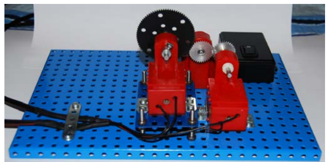
Fig. 3b - Set for measuring the transfer gears
