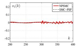
Fig. 20. Evolution of the sliding function  $s_1(k)$ .
