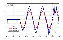
Fig. 12. Evolution of the control signal  $u_1(k)$ .
