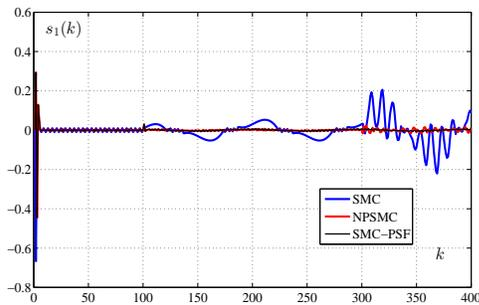
Fig. 14. Evolution of the sliding function  $s_1(k)$ .
