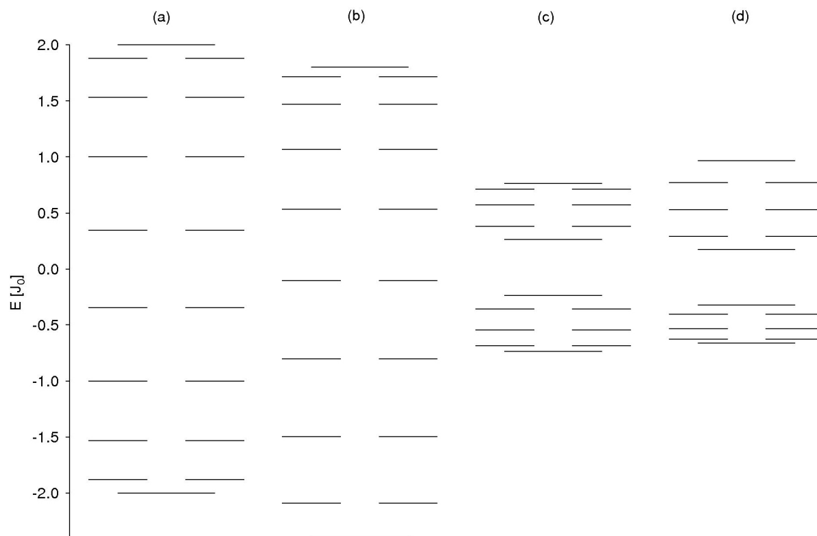
Fig. 1. Energetic band structures for B850 ring from LH2 complex ((a) – the nearest neighbour approximation model, (b) – full Hamiltonian model) and the same for B- \alpha /B- \beta ring from LH4 complex ((c) – the nearest neighbour approximation model, (d) – full Hamiltonian model)
