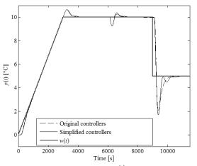
Fig. 8 Simulated control responses of y(t) for the TFC system with controllers (15) vs. (21)
