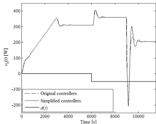
Fig. 7 Simulated control responses of  $u_0(t)$  for the TFC system with controllers (15) vs. (21)
