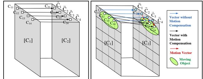
Fig. 3. Definition of vectors  $\bar{C}_s$  for the calculation of the matrix APCA on the basis of  $[C_1]$  and  $[C_2]$ : a - components of vectors  $\bar{C}_s$  without movement compensation; b - components of vectors  $\bar{C}_s$  with block movement compensation.
