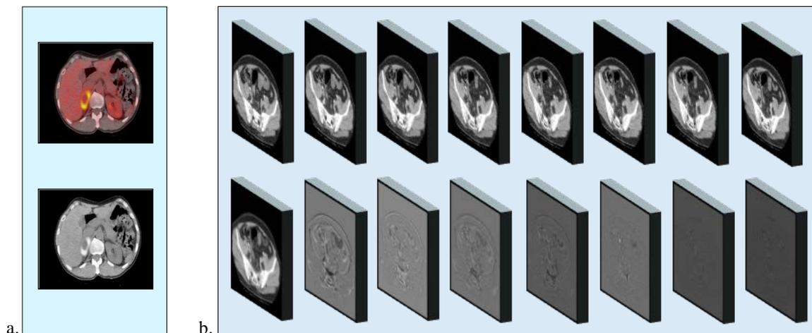
Fig. 7. Example for the double transform of 8 computer tomography images through AC-PCA and HA-PCA
