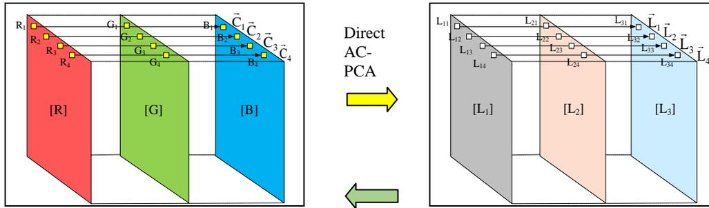
Fig. 1. Transformation of the image RGB components through AC-PCA into corresponding image, which comprises the principal color components L<sub>1</sub>,L<sub>2</sub>,L<sub>3</sub>.
