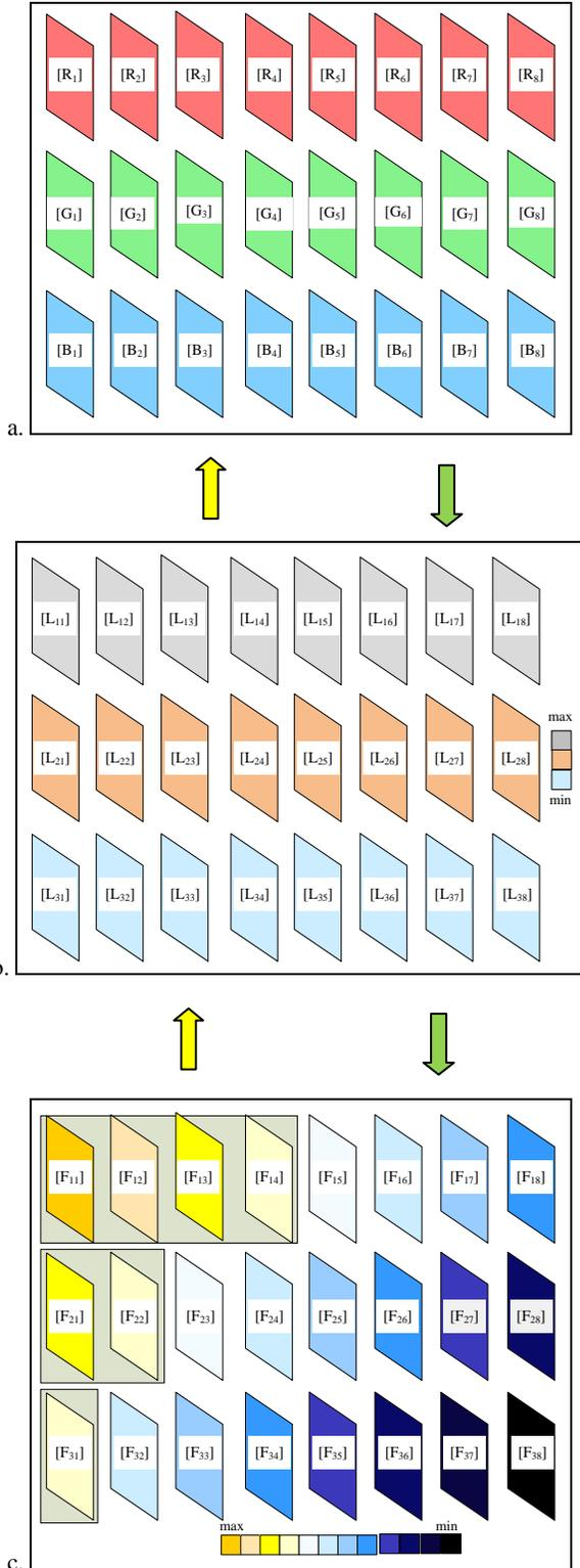
Fig. 6. Double PCA-based transform for a group of 8 RGB images. a - input group of 8 images, represented by their R,G,B components; b - first transform: the AC-PCA is applied on the R,G,B components of each image in the group, and as a result are got three groups of principal components; c - second transform: the HA-PCA is applied on each of the three groups of principal components, got after the AC-PCA transform.
