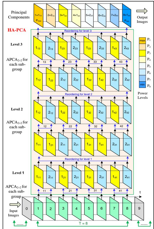
Fig. 5. Hierarchical APCA algorithm for a group of T=8 images, based on the use of APCA<sub>2x2</sub> for each image couple in all three decomposition levels
