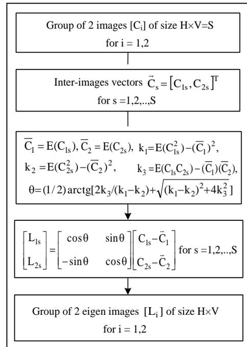
Fig. 4. APCA Algorithm for processing a couple of images
