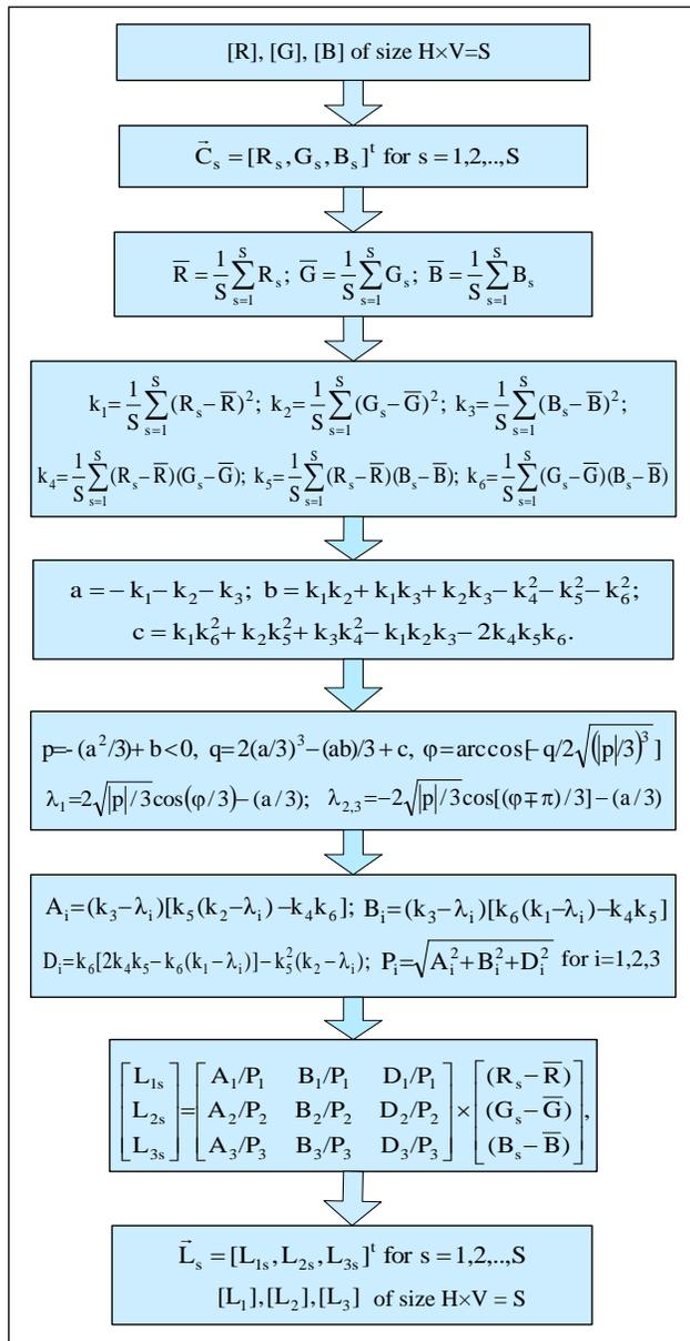
Fig. 2. Block diagram of Algorithm AC-PCA for processing of RGB components
