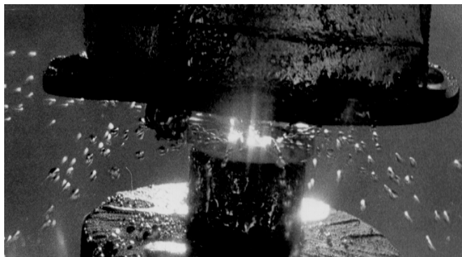
Fig. 2 Electromagnetically controlled resonant film flow decay
