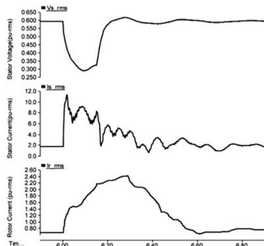
Fig.4 The stator voltage and rotor current without crowbar
