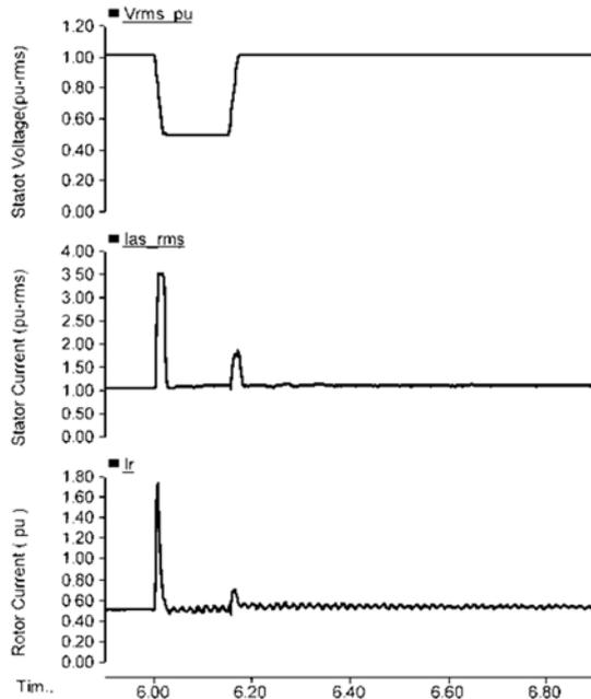
Fig.5 The stator voltage and rotor current with crowbar
