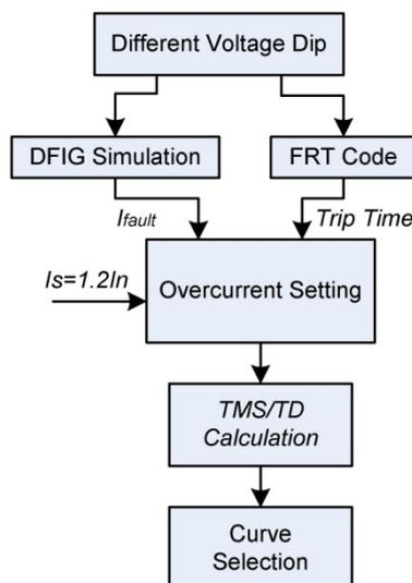
Fig.6 The TMS/TD calculation algorithm
