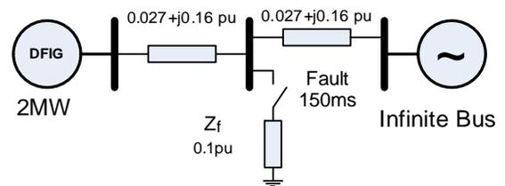
Fig.3 WT-DFIG connection for sag voltage study
