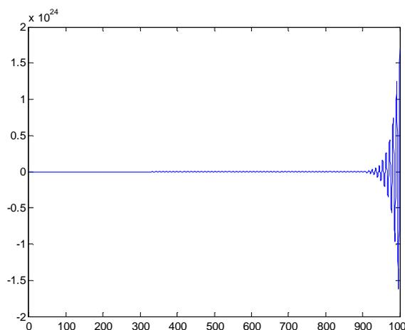
Figure 11: Closed loop step response with PID Controller ( $K_p=0.5$ ,  $K_i=0.05$ ,  $K_d=0.1$ ): unstable case
