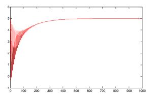
Figure 9: Closed loop step response with PID Controller (Kp= 1, Ki=2.085, Kd=4.2): stable case
