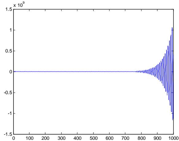
Figure 7: Closed loop response step with PD Controller: (Kp=0.5, Kd=0.4): unstable case
