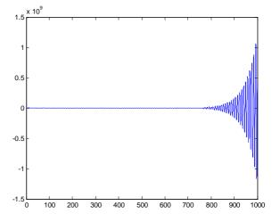
Figure 7: Closed loop response step with PD Controller: (Kp= 0.5, Kd=0. 4): unstable case
