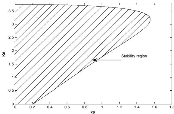
Figure 5: Stability region with PD Controller
