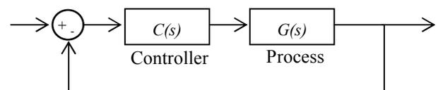
Figure 1: The closed-loop system with controller
