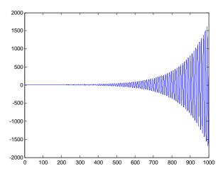
Figure 4: Closed loop step response with PI Controller (Kp= 0.2, Ki=0.04): unstable case
