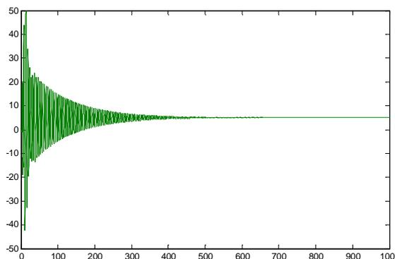
Figure 10: Closed loop step response with PID Controller ( $K_p=0.6$ ,  $K_i=2.085$ ,  $K_d=4.2$ ): stable case
