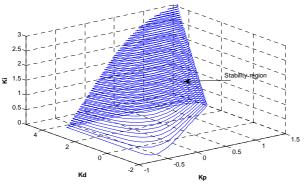
Figure 8: Stability region with PID Controller
