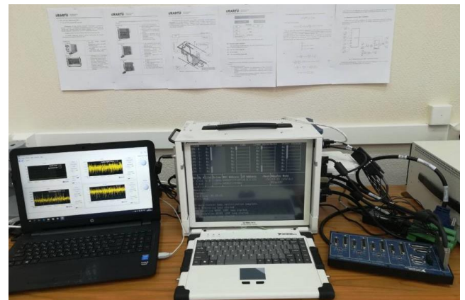
Fig. 3. The HIL US-03 hardware-software stand for simulation of small spacecraft systems.
