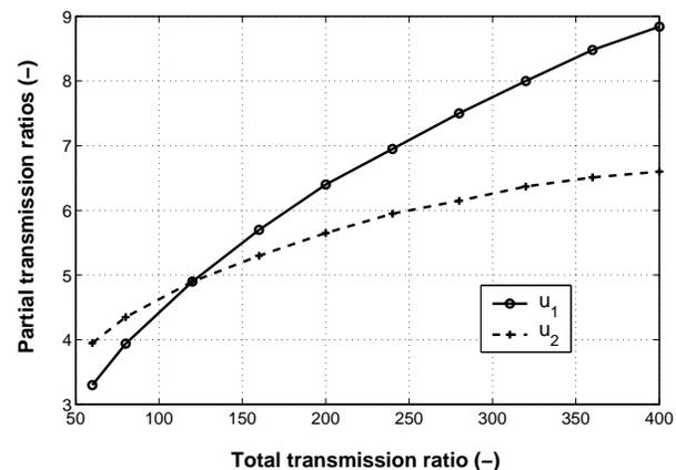
Fig. 1 Determination of the partial ratios of three-step helical gearboxes [1]
