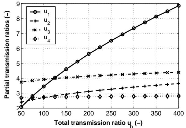
Fig 3: Partial ratios versus the total transmission ratio
