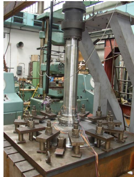
Fig.12 Fatigue testing of railway axles (principles and measurements)
