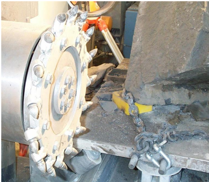
Fig.2 Typical example of mechanical interaction between bits and hard rock (ore disintegration process)
