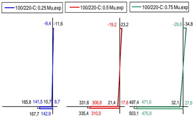
Fig. 6 theoretical (calculated) and actual (derived from the tests) stresses in composite CFRP-timber beam subjected to bending moment: cross-section 100/220-C
