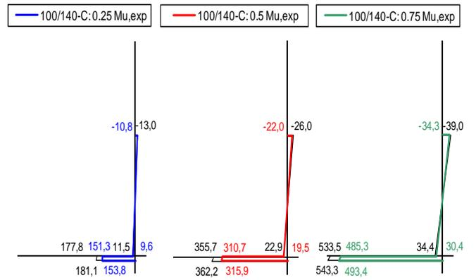
Fig. 10 theoretical (calculated) and actual (derived from the tests) stresses in composite CFRP-timber beam subjected to bending moment: cross-section 100/140-C
