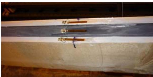
Fig. 5 view to the bottom edge with strain gauges on CFRP lamella and timber surface
