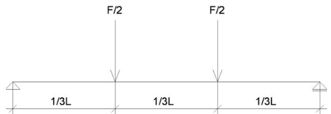
Fig. 2 tested specimen scheme: four-point bending
