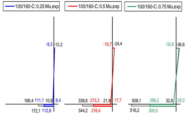
Fig. 9 theoretical (calculated) and actual (derived from the tests) stresses in composite CFRP-timber beam subjected to bending moment: cross-section 100/160-C
