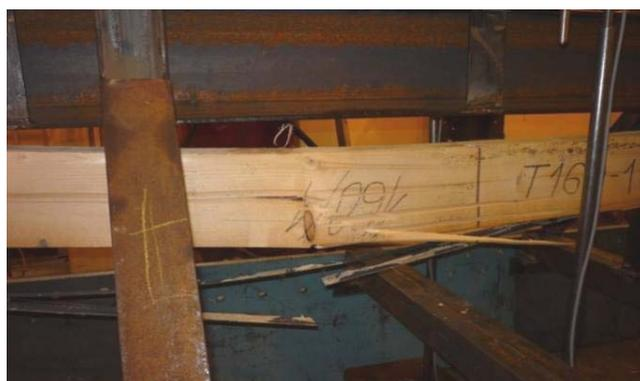
Fig. 12 CFRP lamella rupture together with timber failure
