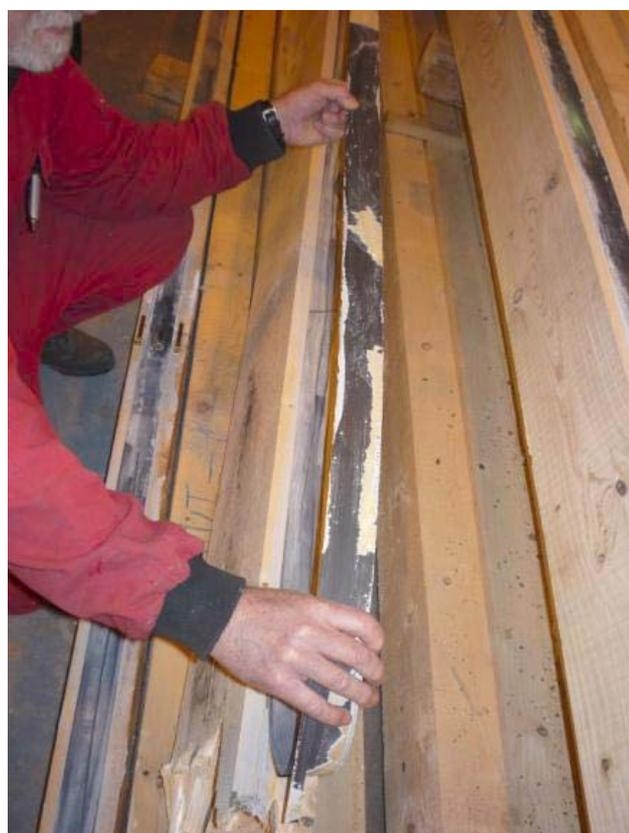
Fig. 14 delaminated CFRP lamella
