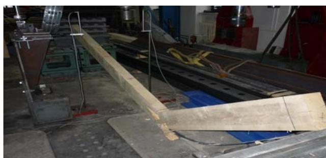
Fig. 13 CFRP lamella separation
