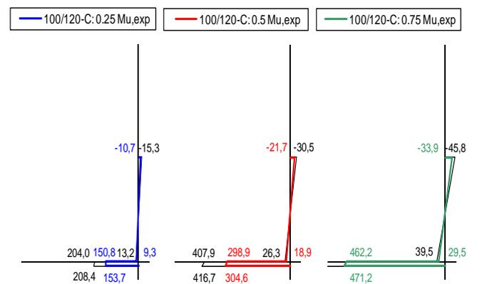
Fig. 11 theoretical (calculated) and actual (derived from the tests) stresses in composite CFRP-timber beam subjected to bending moment: cross-section 100/120-C
