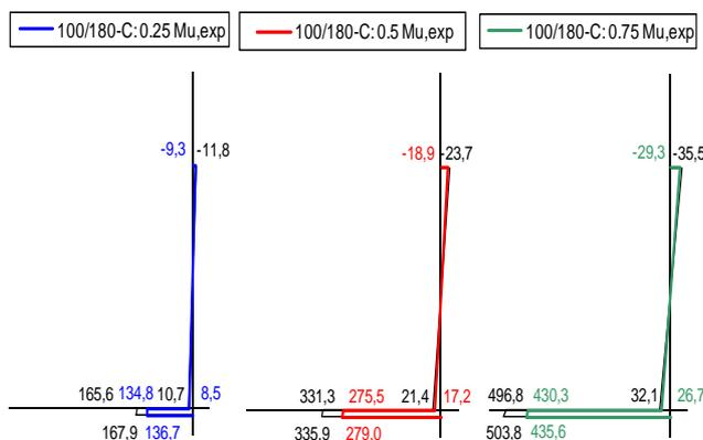
Fig. 8 theoretical (calculated) and actual (derived from the tests) stresses in composite CFRP-timber beam subjected to bending moment: cross-section 100/180-C
