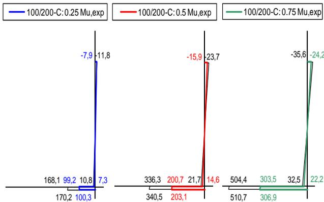
Fig. 7 theoretical (calculated) and actual (derived from the tests) stresses in composite CFRP-timber beam subjected to bending moment: cross-section 100/200-C
