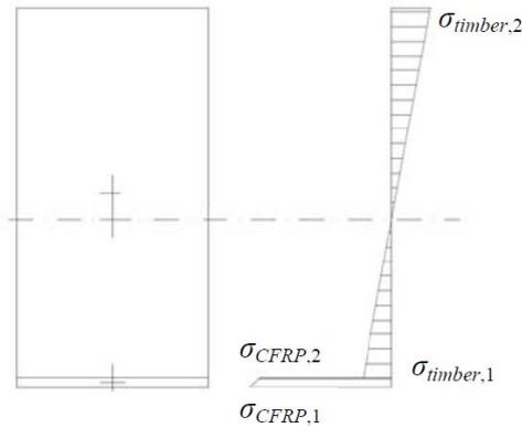
Fig. 1 elastic stress distribution in CFRP-timber beam cross-section
