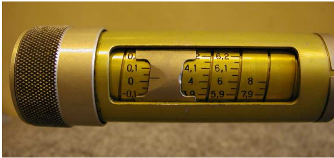
Fig. 4 Reading the value of half segment from PKI-26
