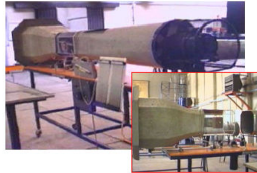
Figure 4. Experimental set: wind tunnel and test section
