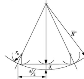
Fig.9 Error caused by linear interpolation for DTC
