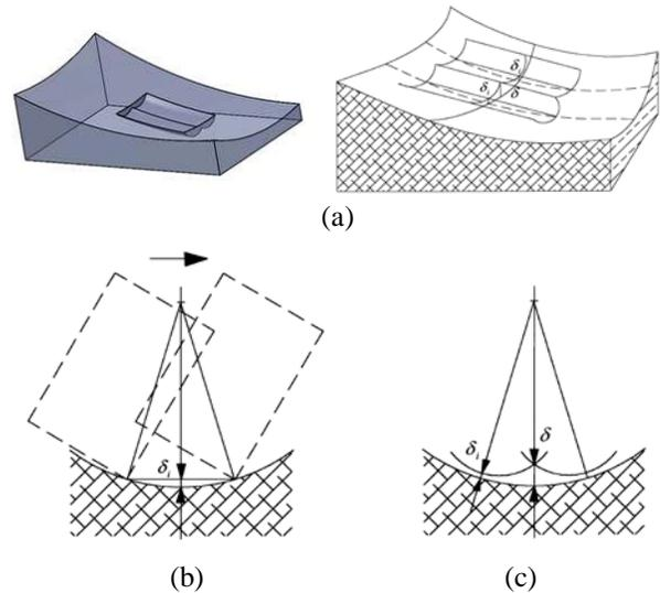
Fig.2 (a) Step-forward linearization and adjacent toolpath, (b)Error caused by the step-forward linearization, (c) Error  $\delta_1$  transmitted into scallop height
