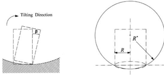
Fig.3 Tilting angle and effective tool radius
