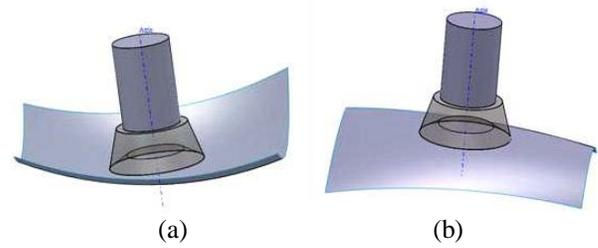
Fig.8 The features of NC machining on the convex and concave elliptical region using DCC
