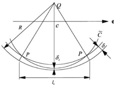
Fig.10 Path interval analysis using envelope
