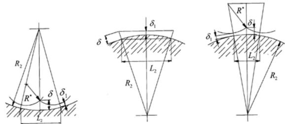
Fig.5 The path interval of flat-end cutter, (a) and (c) the cutter tilts an angle, (b) the axis of cutter aligned with surface normal *Ball-end cutter*
