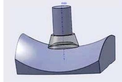
Fig.11 NC machining in hyperbolic region (Saddle like)
