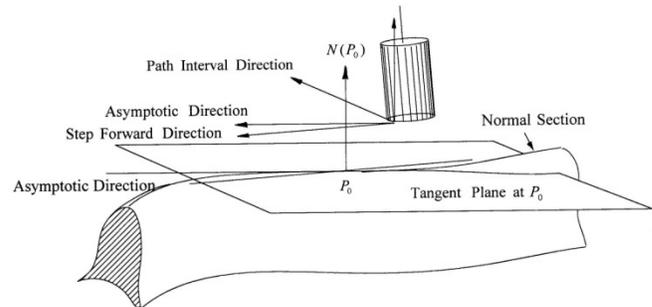
Fig.14 NC machining in parabolic region
