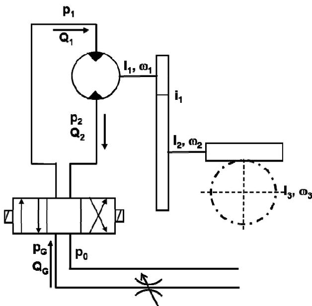
Fig. 10 Hydraulic drive of shell conveyer
