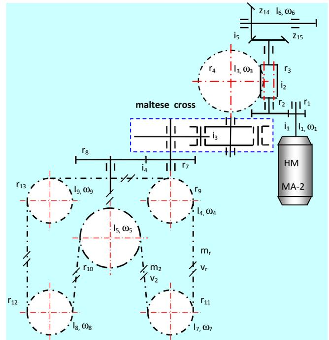
Fig. 3 Kinematic scheme of shell conveyer
