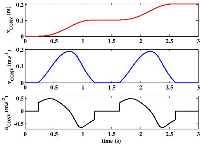
Fig. 12 Kinematic values of shell conveyer
