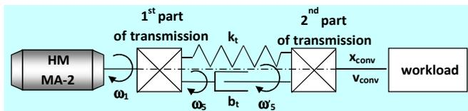
Fig. 18 Flexible binding in dynamic model of shell conveyer
