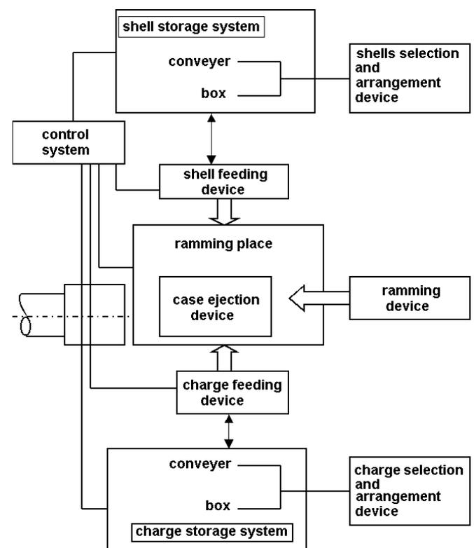
Fig. 1 Loading system of heavy gun scheme
