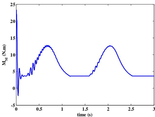
Fig. 21 Torque of hydraulic motor
