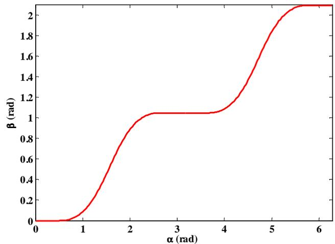
Fig. 6 Maltese cross angular displacement
