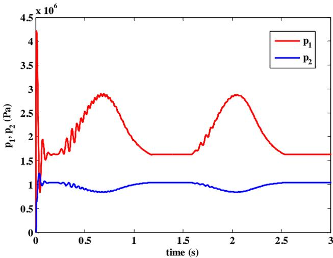
Fig. 20 Input and output pressures in hydraulic motor
