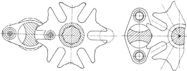
Fig. 4 Maltese cross in and without meshing
