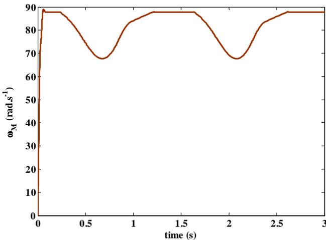
Fig. 13 Angular velocity of hydraulic motor
