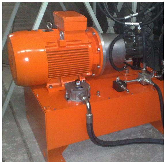
Fig. 23 New hydraulic source
