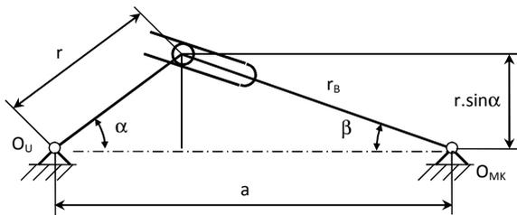
Fig. 5 Kinematics of Maltese cross scheme
