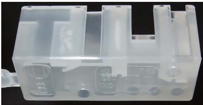
Fig. 16 Defects on part – voiding marks
