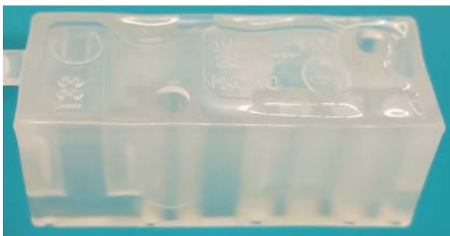
Fig. 17 Defects on part – sink marks
