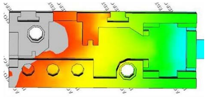
Fig. 19 Defects on part – short shots by simulation
