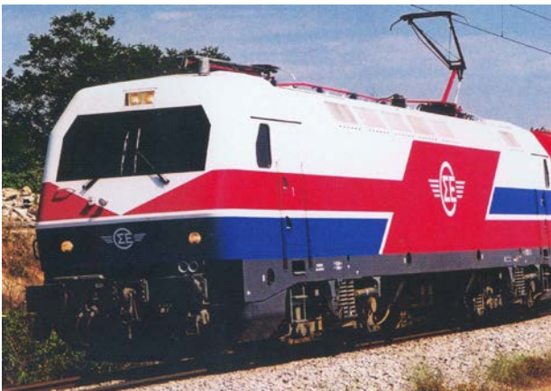
Figure 2 An Electric-Locomotive of the Greek railways with two-axle bogies, on a railway track. The two-axle bogie is marked with the grey ellipses.
