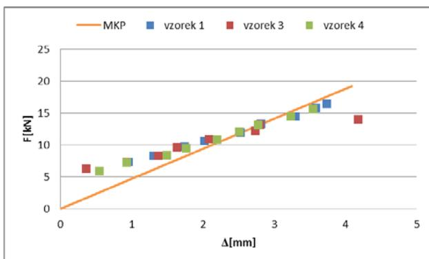
Fig. 7 The comparison of experimental samples without prestress with an MKP model
