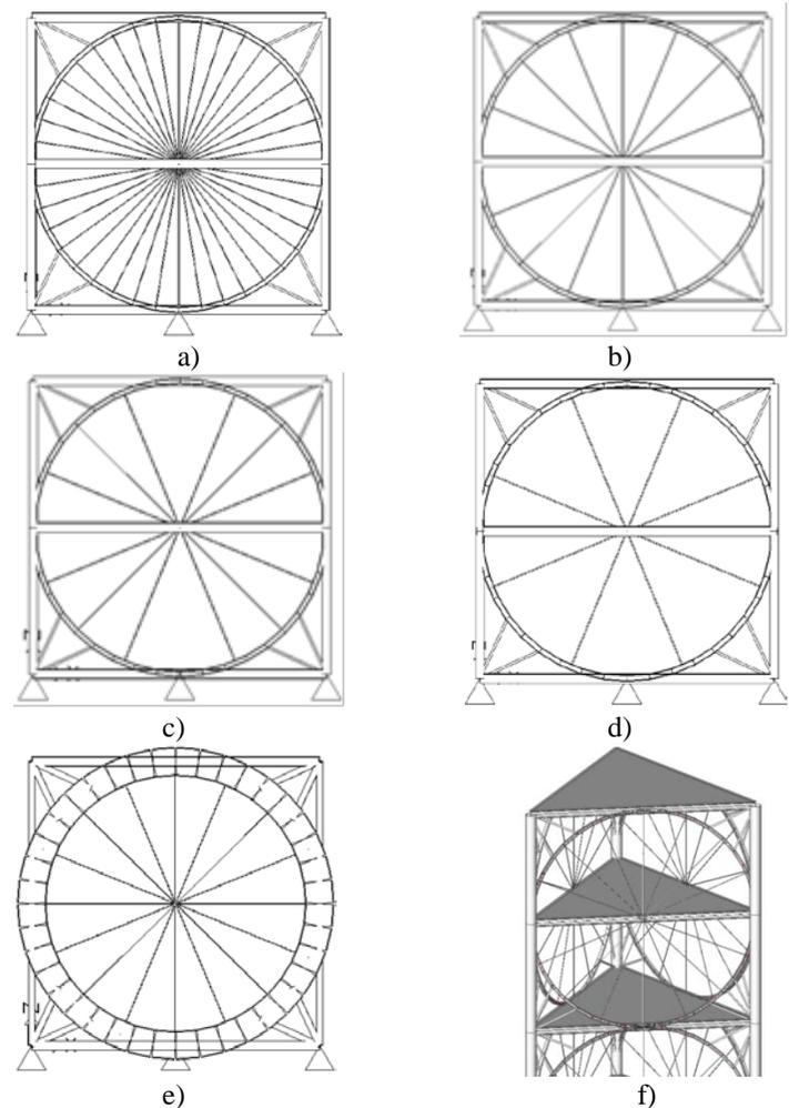
Fig. 1 Hoop wall stiffeners draft schemes a) 40 connecting rods, b) 16 connecting rods, c) 12 connecting rods, d) 8 connecting rods, e) HEA 1000 hoop, f) Stiffener placement construction scheme.
