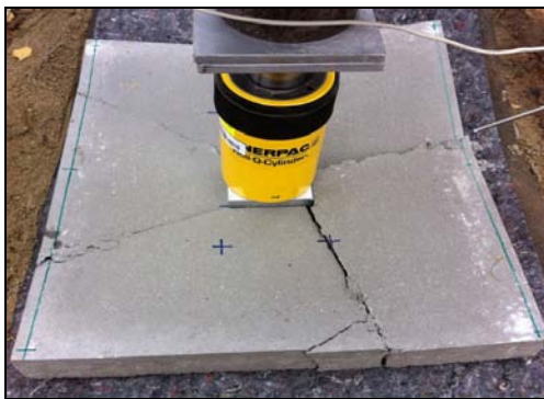
Fig. 4 Failure of the slab
