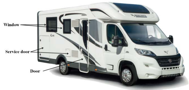
Fig. 1 Typical RV openings [1]
