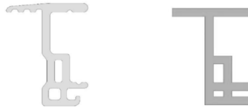
Fig. 18 Comparison between the original (designed) and the simplified bar section of the opening frame.
