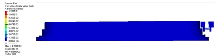
Fig. 26 Von Mises stresses induced in the most critical step of the slam test
