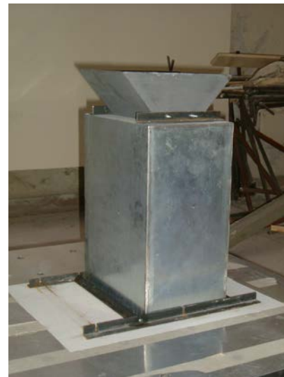
Fig.4 – Sample of dynamic tests on purely rocking blocks equipped with a trapezoidal TLD, fixed on the top.
