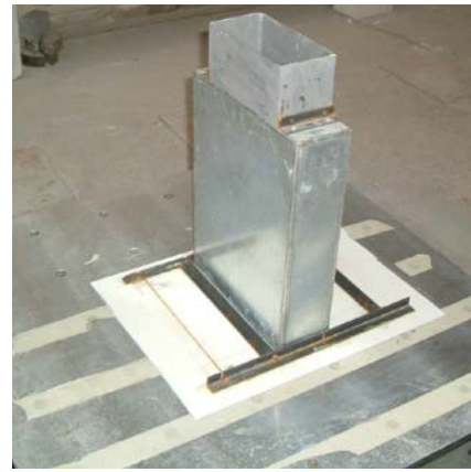
Fig.3– Sample of dynamic tests on purely rocking blocks equipped with a rectangular TLD, fixed on the top.
