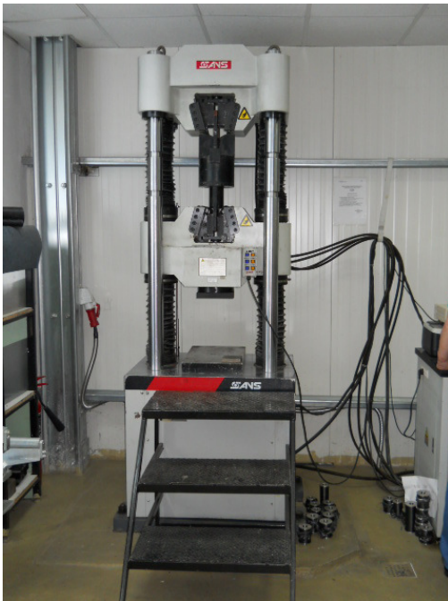
Fig. 30 Testing the SERB 3 damper on SANS testing machine at ICECON laboratory
