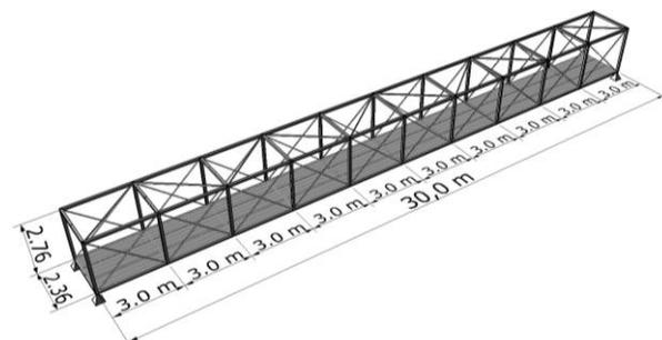
Fig. 1 basic dimensions of the developed "long" footbridge
