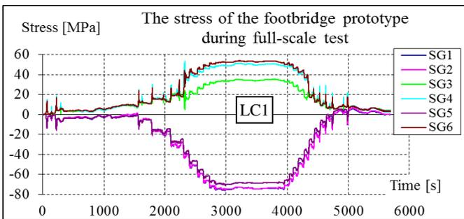
Fig. 20 the values of the stress (for strain gauges SG1 to SG6)
