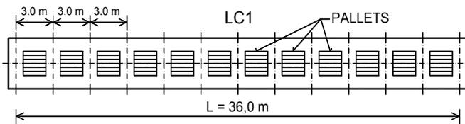
Fig. 15 the scheme of the arrangement of pallets (1 pallet = 1000 kg)
