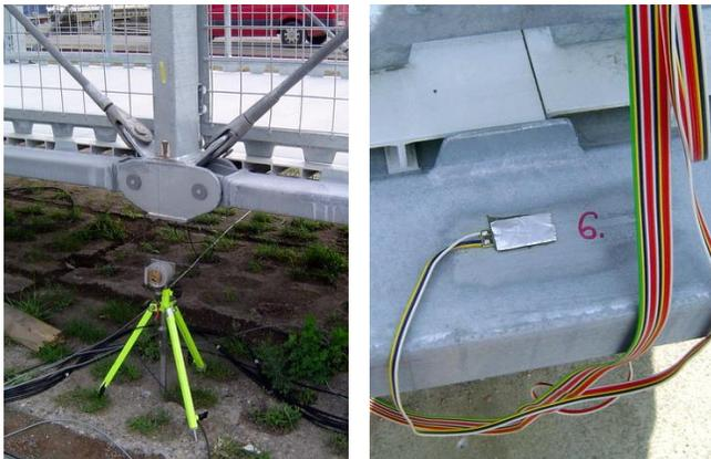
Fig. 14 an example of used potentiometric sensor of deformations (left) and an example of used strain gauge (right)
