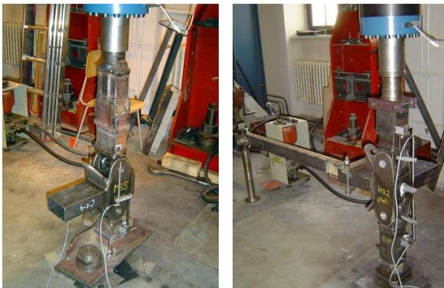
Fig. 6 the illustration of static loading tests with the tension (left) and compression axial force (right)
