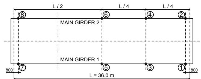
Fig. 12 the positions of the potentiometric sensors of deformations
