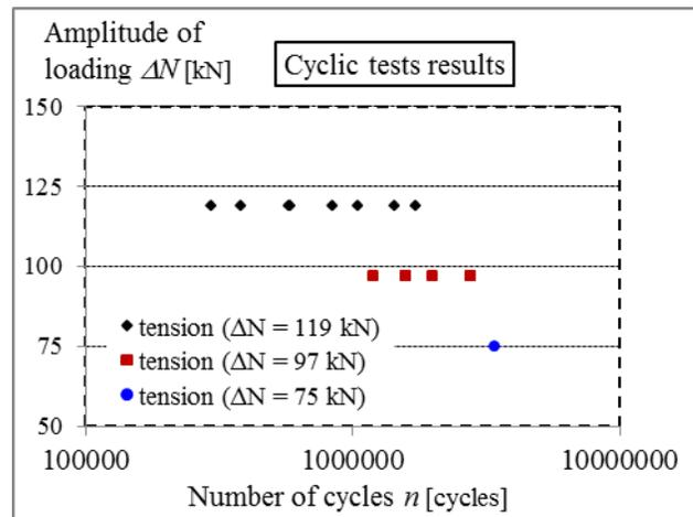
Fig. 10 the results in case of cyclic tests using tension force
