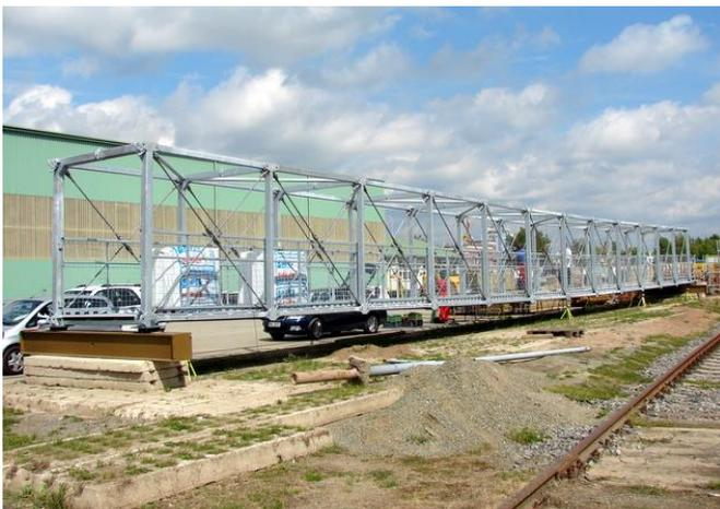
Fig. 3 the footbridge prototype used for full-scale testing
