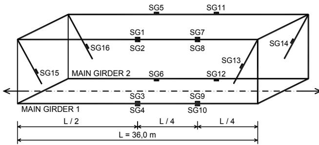
Fig. 13 the positions of the strain gauges
