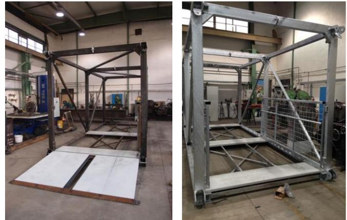
Fig. 11 prepared assembly units before (left) and after a galvanization
