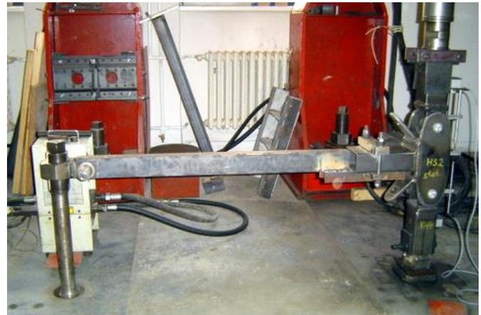
Fig. 7 the additional support of the specimen in case of the static loading test with use of a compression axial force
