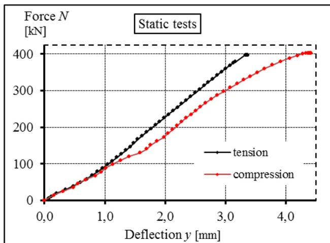
Fig. 5 the force-to-deflection relationships in case of static tests
