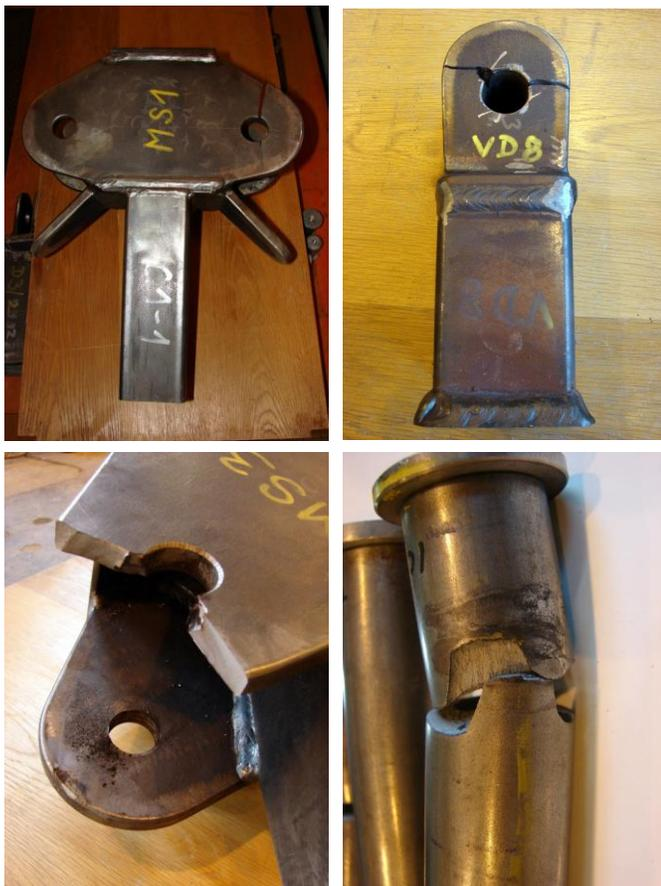
Fig. 8 the illustration of the failed specimens in case of tension and compression joints under repeated loading (failed splice plate of the middle part – top and bottom left, failed splice plate of the end part of lower chord – top right, failed pin – bottom right)
