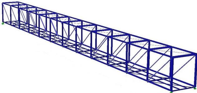
Fig. 2 the original FEM model of the footbridge
