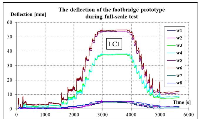
Fig. 18 the deflection-to-time relationships of the footbridge prototype in case of distributed load
