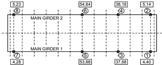
Fig. 19 the values of the deflection in case of distributed load
