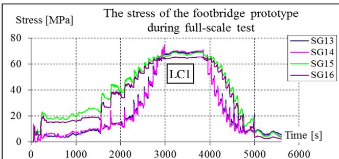
Fig. 22 the values of the stress (for strain gauges SG13 to SG16)
