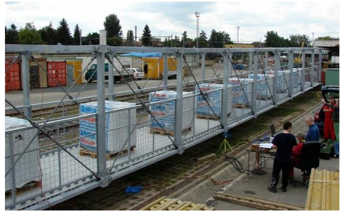
Fig. 17 the final state in case of the uniformly distributed load
