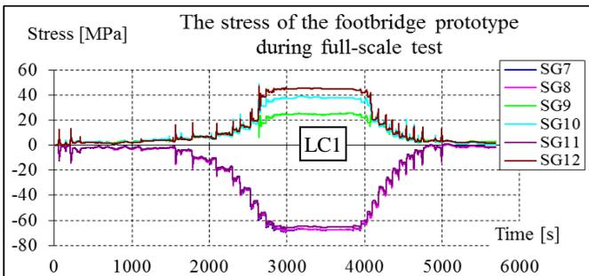
Fig. 21 the values of the stress (for strain gauges SG7 to SG12)
