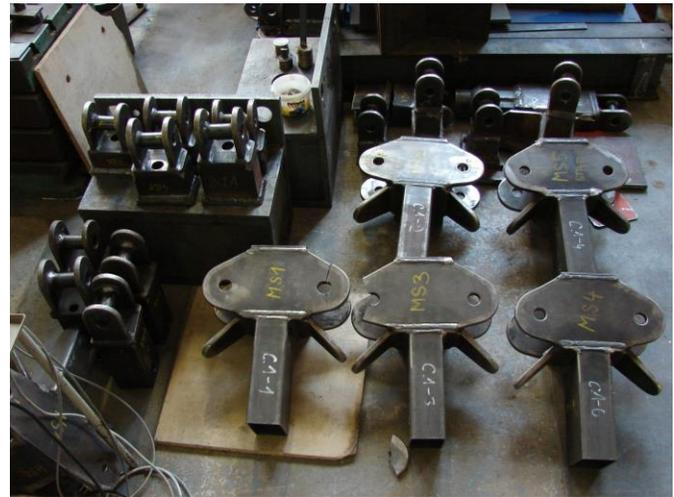
Fig. 9 the failed specimens of the temporary footbridge joints
