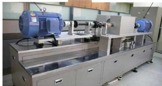
(a) side view of the scaled adhesion test-bench
