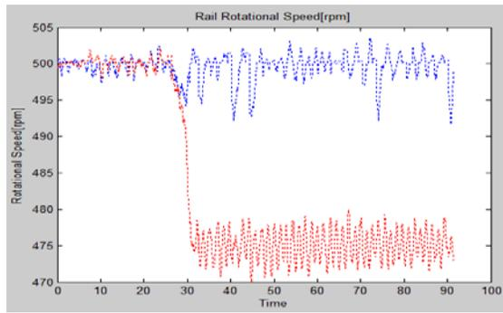
(a) rotational speed of wheel disc and rail disc
