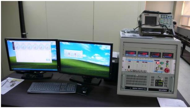
(c) control console for the scaled adhesion test-bench
