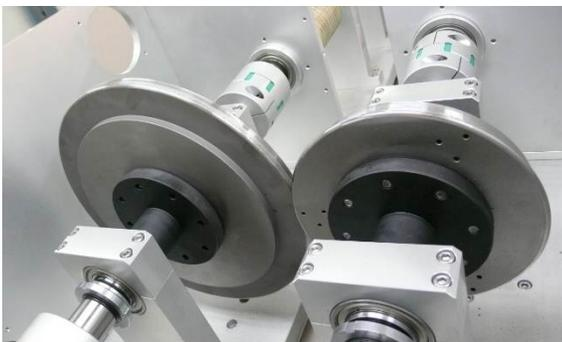
Fig.4 specimens of wheel and rail for the scaled adhesion test-bench
