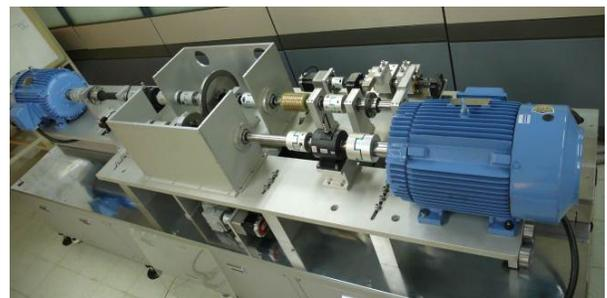
(b) upper side view of the scaled adhesion test-bench
