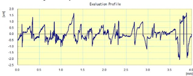
Fig. 6 surface roughness profiles of the rail spacemen at the initial state
