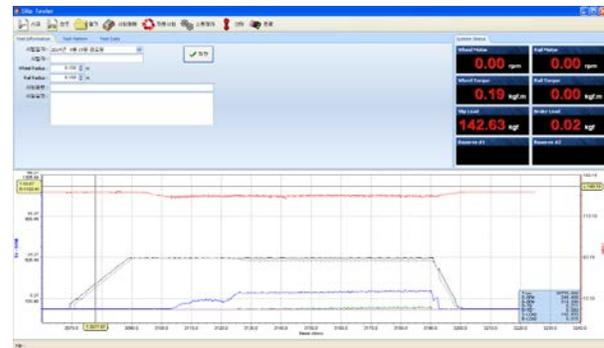
Fig.13 Experimental environments: wheel and rail speed, torque, and axle load
