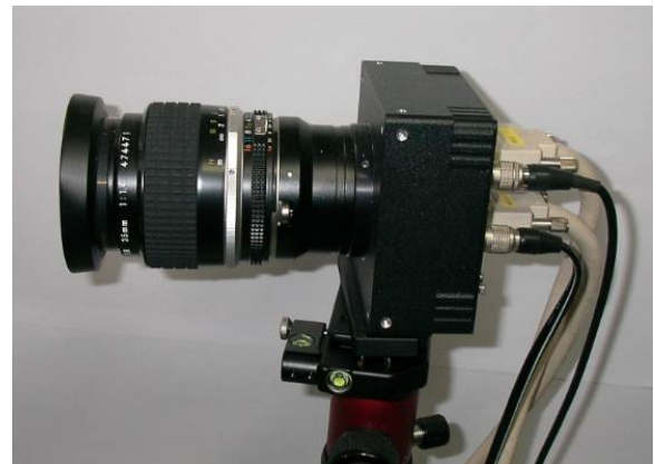
Fig.5 the high speed camera for analyzing the temperature transition of the disc surface
