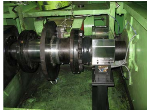
(b) disc brake parts of the brake dynamometer
