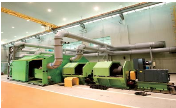
(a) drive motor and inertia parts of the brake dynamometer
