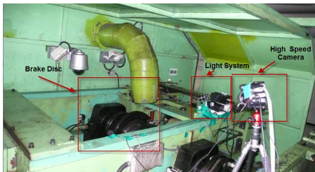
(a) experiment device is made up of three parts: the brake disc, the light systems, and the high speed camera
