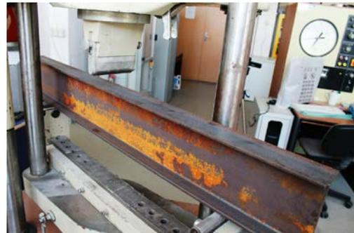
Fig. 8 three-point bending test on IPN 160 – experiment.
