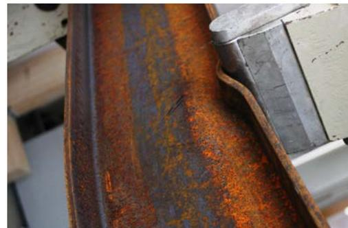
Fig. 9 failure in the beam - web buckling.
