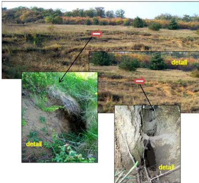
Fig. 3 Break points zone on the subsidence edge of the undermined territory Kosice-Bankov; red arrow – the zones of break points
